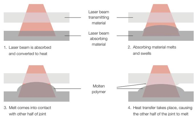
Fig. 1: Schematic description of the transmission welding process
