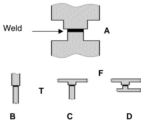
Figure 3. Welded joint design basics. Agenda: A—standard; B—straight; C—T-type; D—shear/lap; E—flange (T-type joint); T – vertical wall/plaque.
