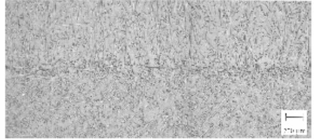
Figure 10. An example of glass-fibers re-orientation at weld inter-phase (melt-pool) for 33 wt.% short fiber-glass reinforced nylon 6. A part of glass-fiber is crossing inter-phase at optimized welding conditions.
