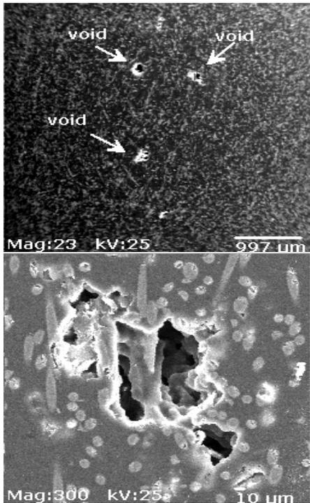
Figure 11. An example of micro-voids formation during non-optimized injection molding of glass-fiber reinforced thermoplastic
