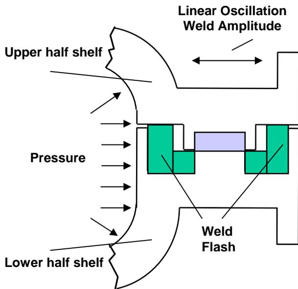
Figure 8. Butt-joint design principles for automotive linear vibration welded hollow components [1, 13-14].
