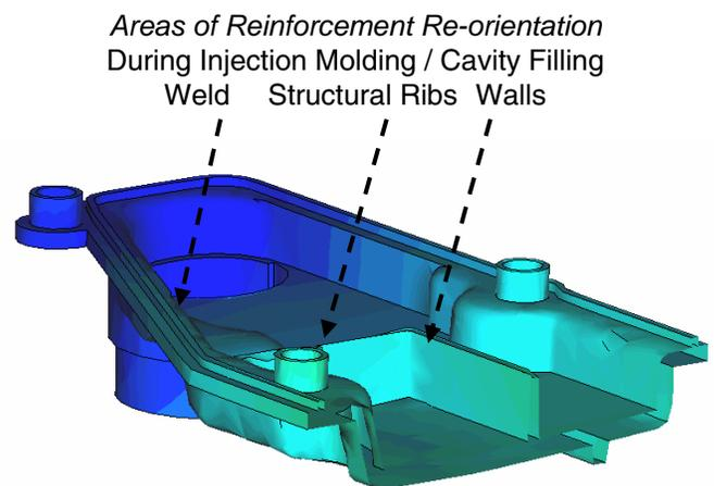
Figure 2. Example of Moldflow<sup>®</sup> simulation for injection molded part (for details see Figure 1). Range of color shades indicate filling time, i.e., dark blue=start.
