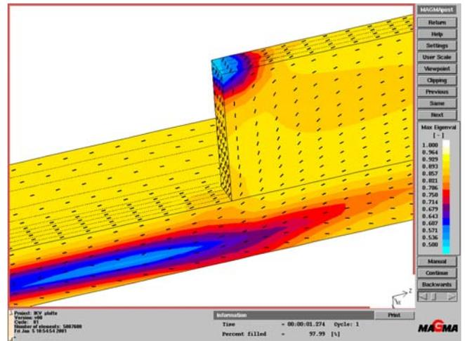
Figure 12. SigmaSoft™ analysis close-up plot showing predicted fiber orientation through thickness. Fiber principle direction is indicated by the black lines. Degree of orientation is shown with color-bar<sup>13</sup> on right—yellow (light) indicates highly aligned, blue (dark) is random.
