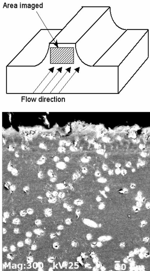
Figure 9. Glass-fiber orientation at injection molded “tooth” area of weld bead (for 33 wt.% short fiber-glass reinforced nylon 6)
