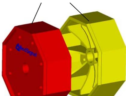
Figure 7. Multi-purpose universal welding & testing system (Consists from welded together two octagonal specimens [15]. Thickness of weld beads may vary from 2.5 to 6 mm. U.S. Patent # 6,193,133).
