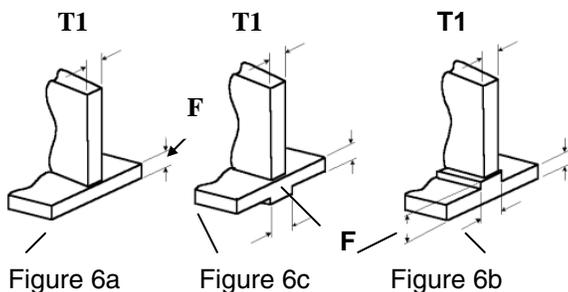
Figure 6 (a, b, c). Principles of T-type joint geometry (a – similar by thickness parts, b – with T-shape weld-bead, c – reverse position of Tr-shape weld-bead). F is the thickness of T-element at the future joint area.
