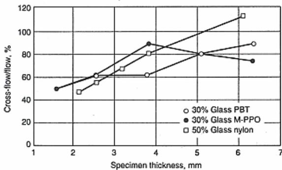
Figure 14. The influence flow direction, part/specimen thickness on mechanical performance of injection molded glass-fiber reinforced thermoplastics (nylon, PBT and M-PPO based) [1].
