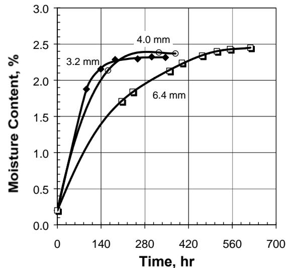
Figure 11. Moisture absorption (in wt.%) vs. time for 33 wt.% glass fiber reinforced nylon 6 with various walls thickness (mm): 3.2; 4.0; 6.25.
