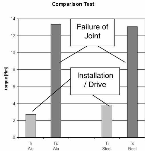
Figure 20. Influence of used fasteners on installation and ultimate conditions of assembly (Delta 60, number of engaged threads = 4).
