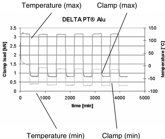
Figure 21. Influence of time-temperature effects on the kinetic of clamp load for aluminum made fastener.
