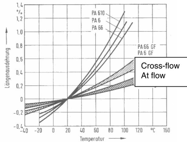
Figure 17. Influence of temperature on thermal expansion of the various nylons [36].
