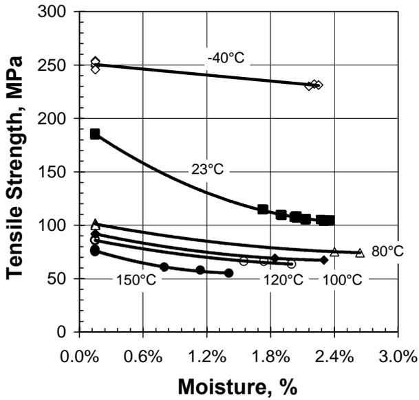
Figure 12. Influence of end-use temperature and moisture on the tensile strength of reinforced nylon 6 (33% short glass-fiber).
