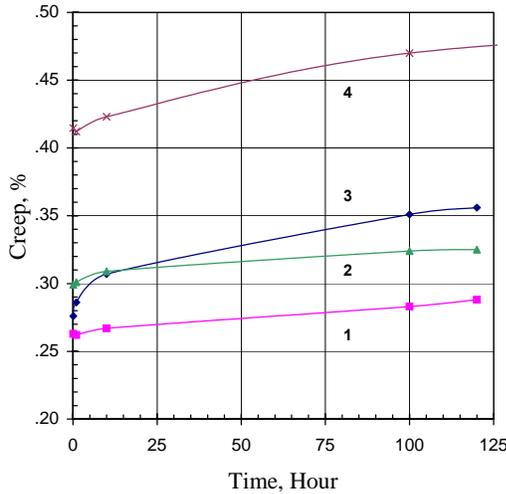
Figure 15. Influence of reinforcement type on resistance to tensile creep of nylon 6. Legend: material state: DAM, color - natural state; Test temperature - 23°C; 1 - 63 wt.% GF; 2 - 50 wt.% GF; 4 - long fiber-glass (50 wt.% GF); 4 - 33 wt.% GF.
