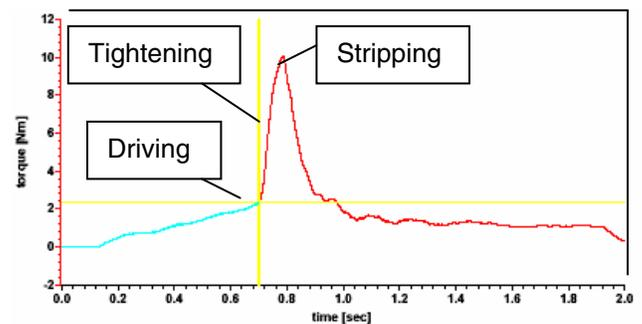
Figure 19. Relations between torque and tightening time (rotation of self-tapping screw).
