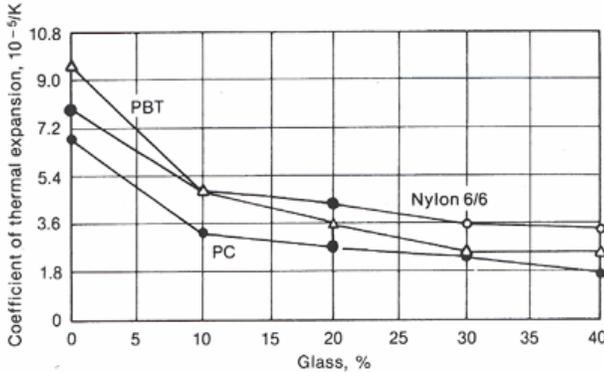
Figure 16. Influence of fiber-glass reinforcement on linear thermal expansion of three thermoplastics (nylon 66, PBT, and PC based, at 23°C, dry-as molded)
