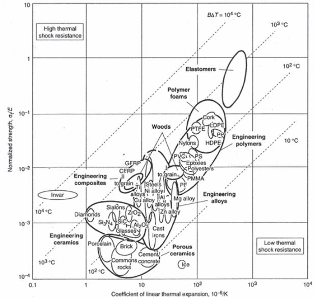
Figure 6. Relations between the linear thermal expansion ( $\alpha$ ) and normalized strength ( $\sigma/E$ ).
