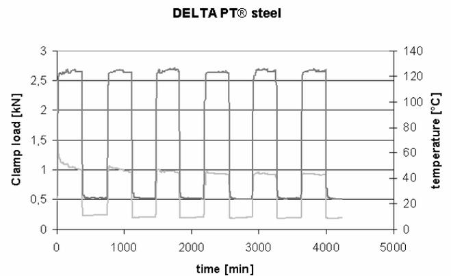
Figure 22. Influence of time-temperature effects on the kinetic of clamp load for steel made fastener.
