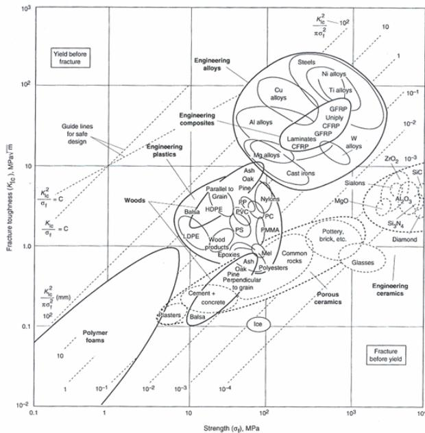
Figure 9. Relations between material tensile strength ( $\sigma_u$ ) and fracture toughness ( $K_{IC}$ ).
