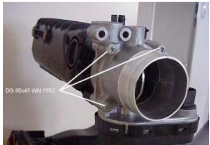
Figure 1. An example of the assembly (fastening technology) of the plastic part and metallic component.
