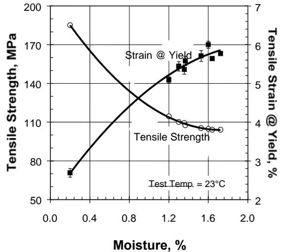
Figure 14. The effect of moisture on tensile properties of short glass-fiber reinforced nylon 6 (33 wt.%): Tensile strength and strain at yield vs. moisture at  $23^{\circ}\text{C}$ .
