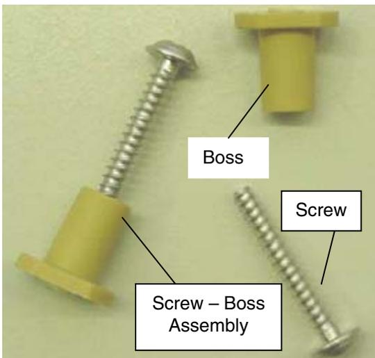
Figure 19. Test modes/specimens (an injection molded boss and self-tapping screw – Delta 60).
