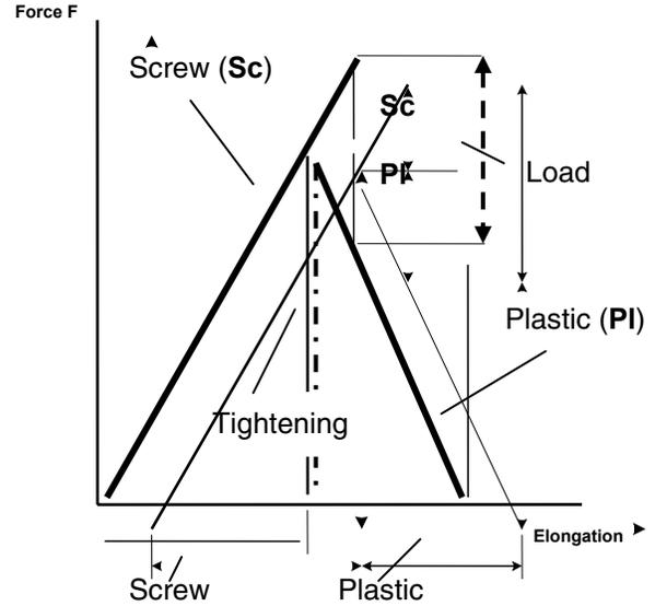
Figure 8. Loading diagram for a plastic-screw joint
