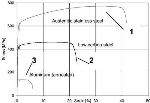
Figure 5. Tensile stress-strain curves for two grades of steels (1-2) and aluminum (3) for fasteners applications.
