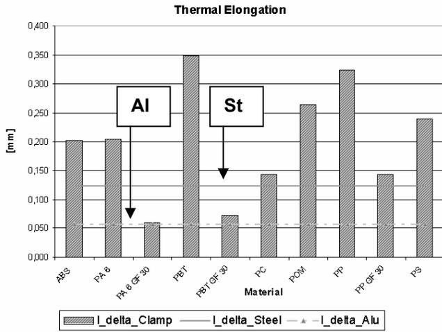
Figure 7. Relations between the linear thermal expansion  $\alpha$  of various thermoplastics and thermal elongation of self-tapping screws (aluminum - **AI** and steel - **St** made) for unconstrained conditions.
