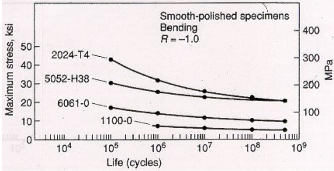
Figure 18. Flexural fatigue data: S-N curves for analyzed aluminum alloys (1100 – annealed; 2024 – strain-hardened; 6061/6063 - strain-hardened) at 23°C, symmetrical stress cycle  $R = -1$ .
