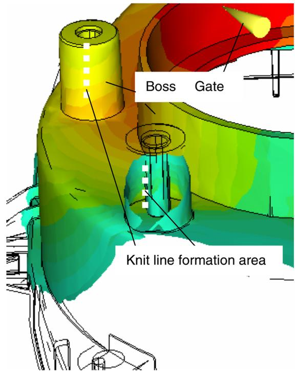
Figure 10. Plastic flow patterns in boss area with knit-line formation (MoldFlow® data).
