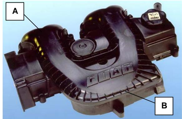
Figure 11. Plastic air intake manifold (potential “dream application of the author’s” for through-transmission laser welding technology). Legend: A – top part molded from laser transparent polyamide 6 colored in black; B – base part colored by carbon black (laser energy absorber).
