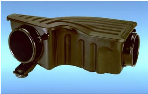
Figure 23. Vibration welded plastic resonator (injection molded from PA 6 colored in black, potential application for through-transmission laser welding technology).
