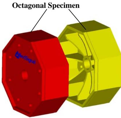
Figure 8. Multi-purpose universal welding & testing system (Consists from welded together two octagonal specimens. Thickness of weld beads may vary from 2.5 to 6 mm).
