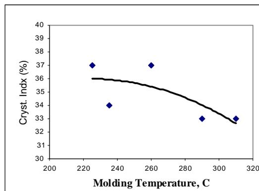
Figure 14. Influence of molding/melt temperatures on CI (crystallinity index).
