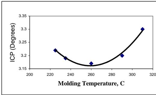
Figure 15. Influence of molding/melt temperatures on ICP.
