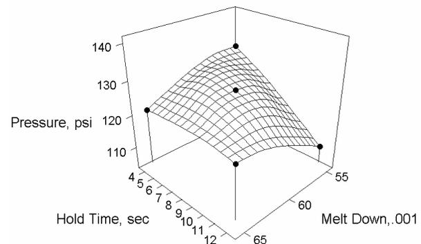
Figure 11. Example of Welding Process and Design Optimization: Burst Pressure Data for Vibration Welded AIM [14].
