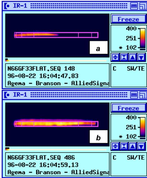
Figure 12. Temperature distribution in the weld inter-phase for butt joint, PA 66, 33 wt.% GF. Legend: **a** - heating initiation phase; **b** - at final phase of heating.
