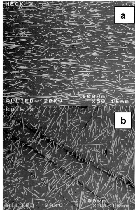
Figure 1. Fiber-glass orientation in injection molded ISO 3167 multipurpose specimen (PA 6, 33 wt.% GF): **a** – fiber orientation at flow direction in narrow parallel-side portion, **b** – fiber orientation in “end”/gate portion.
