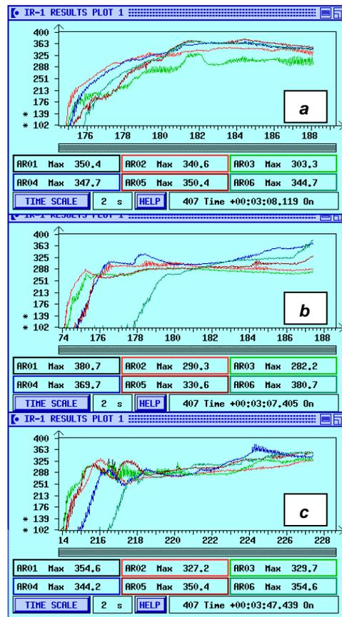
Figure 13. Time-temperature profiles (optimized LVW conditions, butt joint, and PA 66). Legend (type of used plastics): **a** -- non-reinforced/non-filled; **b** - 33 wt.% fiber-glass reinforced; **c** - fiberglass reinforced and mineral filled.
