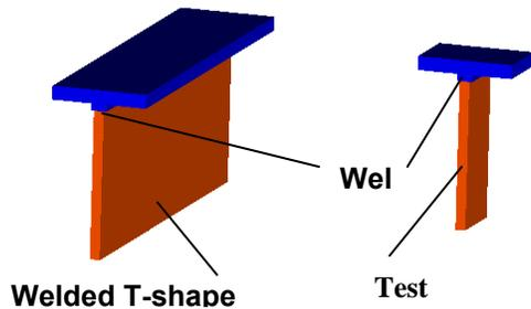
Figure 6. Mode of welded T-shape butt joint (consists from welded together T-element and molded plaques. For T-element thickness of the weld bead is 6 mm. Thickness of the plaque is 4 mm) and machined/cut T-shape test specimen (width = 10 mm). Thickness of the weld beads may vary from 1.6 to 6.25 mm.
