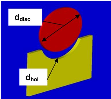
Figure 9. Curvilinear mode of the welded joint (injection molded disc and plaque will be joined together by linear vibration welding). Thickness of weld beads may vary from 1.6 to 6.25 mm.
