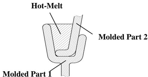
Figure 16. Principles of Hot-Melt joining (over-molding)
