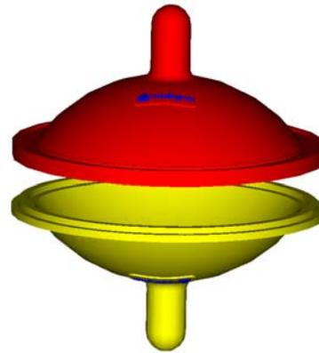
Figure 10. Two Shelves Model. Thickness of weld beads may vary from 2.5 to 6 mm.
