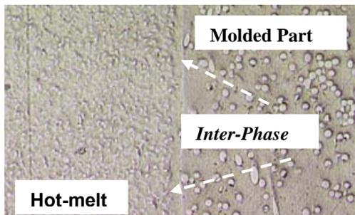
Figure 17. Joint Structure at Optimized Over-Molding Conditions
