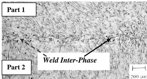
Figure 2. Local reinforcement effects at the weld inter-phase (a part of fibers are crossing the weld inter-phase). PA 6, 33 wt.% GF.
