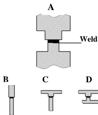
Figure 3. Welded joint design principles (types and configuration). Legend: **A** – joint design; **B** – butt joint (straight); **C** – butt joint (T – shape); **D** – shear/lap joint.
