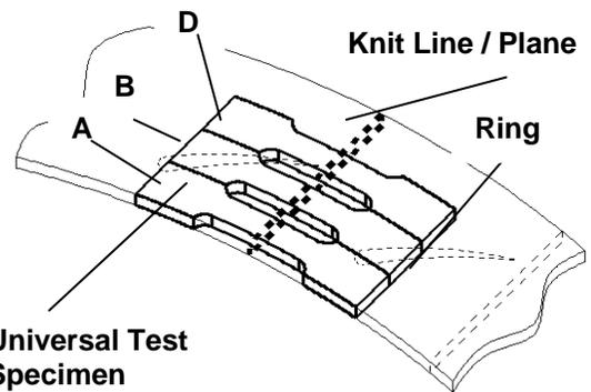
Figure 20. Experimental evaluation of tensile strength at the knit line/plane on the universal test specimens cut from a ring
