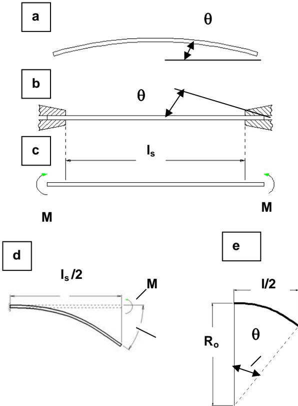
Figure 22. Experimental evaluation of strength at knit-line (plane) – testing of cut specimen with initial curvature.
