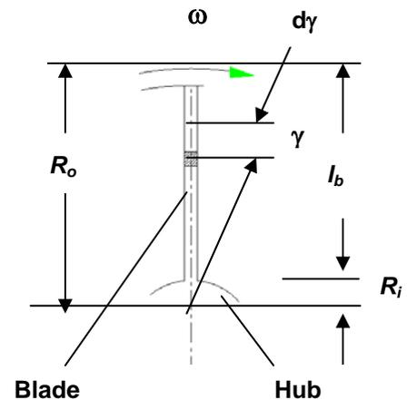
Figure 12. Blade rotating on a rigid metallic hub
