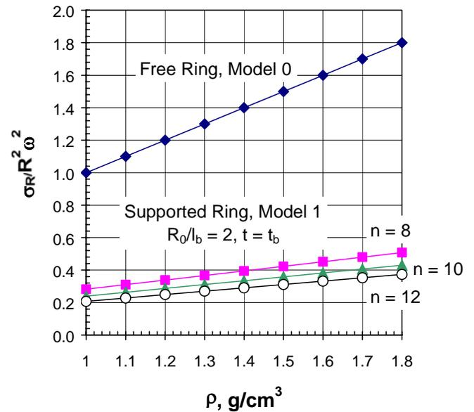
Figure 13. Normalized stress ( $\sigma_R / R^2 \omega^2$ ) as a function of thermoplastic density  $\rho$
