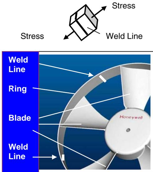
Figure 7. Weld lines formation in a ring of cooling fan (between every pair of the blades)
