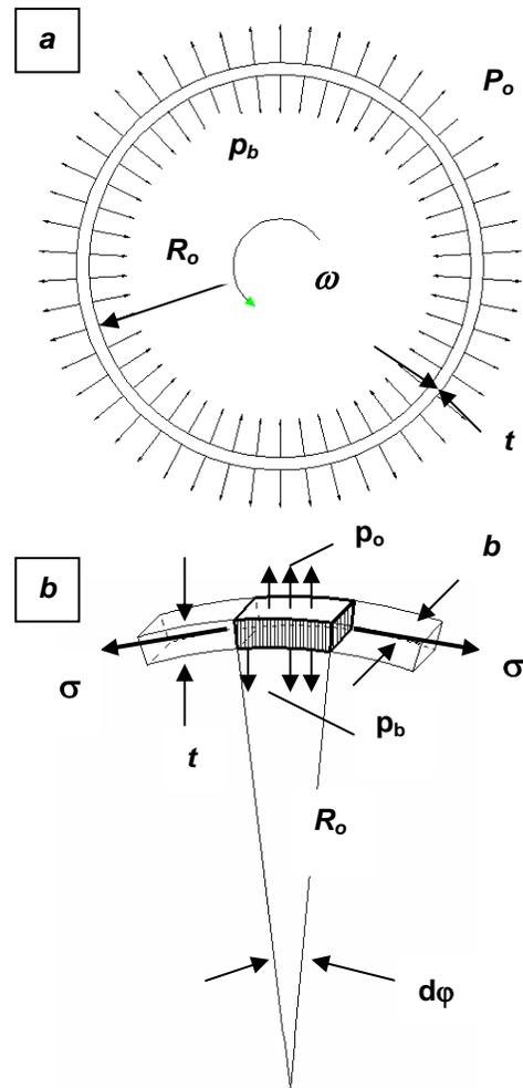
Figure 10. Rotating ring and the loading scheme (Model 0)
