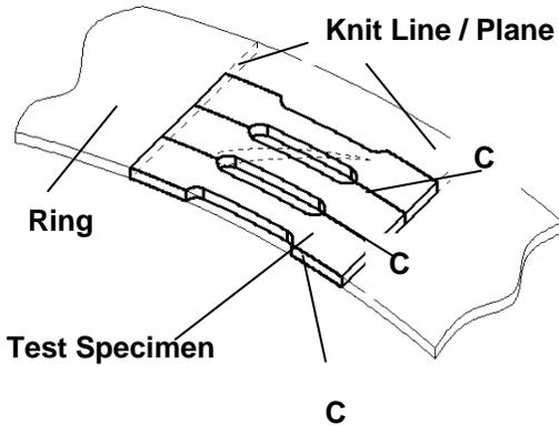
Figure 21. Experimental evaluation of tensile strength at the bulk area (out of the knit-lines) on the universal test specimens from a ring
