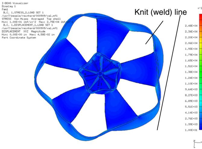
Figure 17. Structural design optimization study: An example of the radial displacements/deflections distributions for cooling fan with a ring (FEA data)
