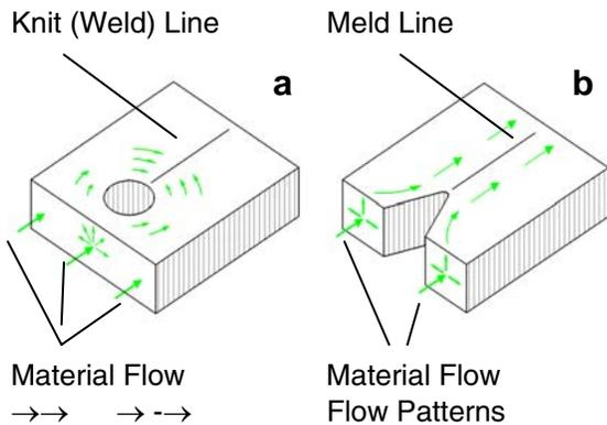
Figure 4. Principles in formation of knit (weld) and meld line and weld & meld flow paths: a – flow around cylindrical hole; b – flow around ribs or long insert.
