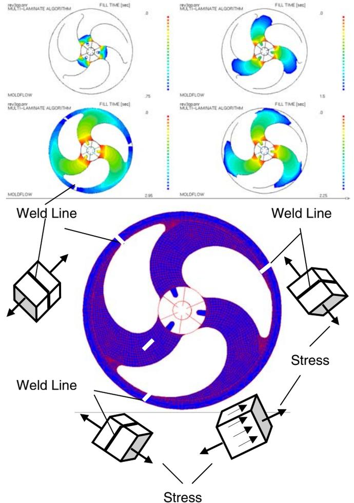
Figure 6. Flow patterns and weld lines formation (MoldFlow® data) in the injection molded thermoplastic part with a ring (nylon 6, 33 wt.% GF)
