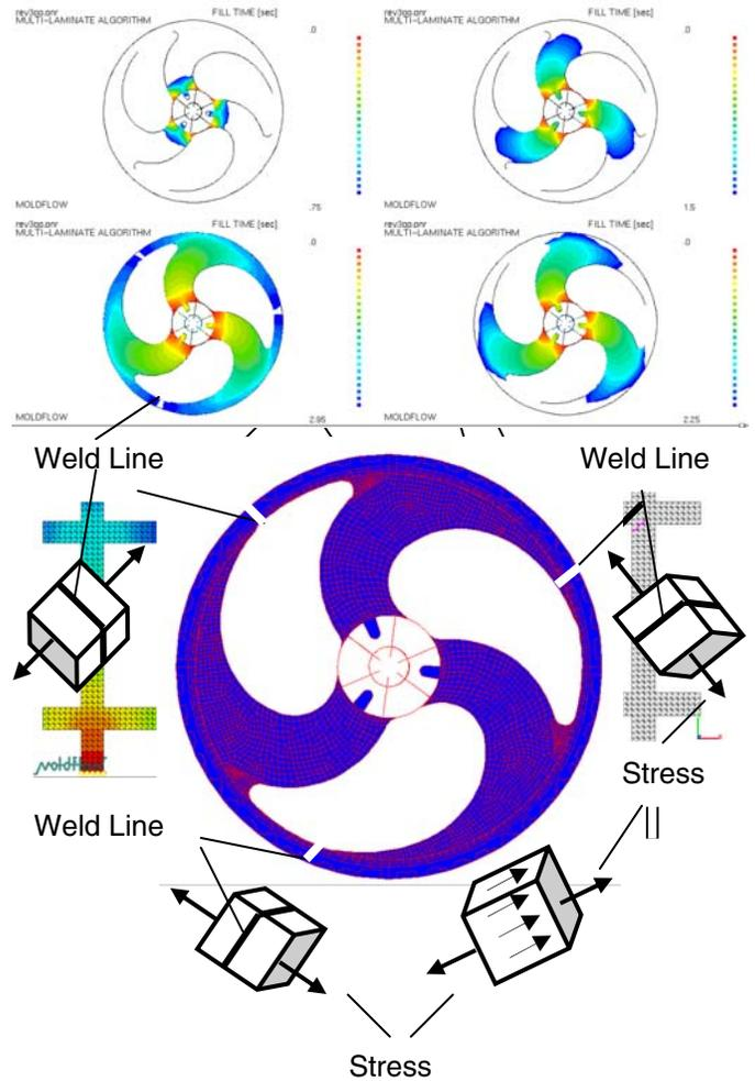
Figure 9. Different plastic flow patterns create weld and meld lines (MoldFlow® data)
