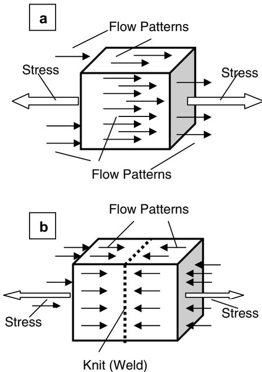
Figure 8. Effect of orientation on mechanical performance of injection molded parts/specimens: a – applied stress is parallel to flow direction (unidirectional fiber-glass orientation); b – applied stress is perpendicular to the knit (weld) line.
