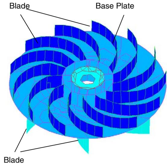
Figure 10: Structural model of injection molded multi-blade impeller
