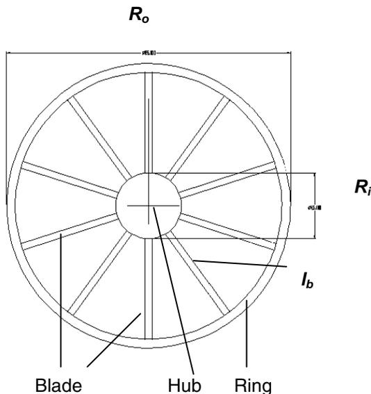
Figure 11. Ring with the blades and a rigid metallic hub
