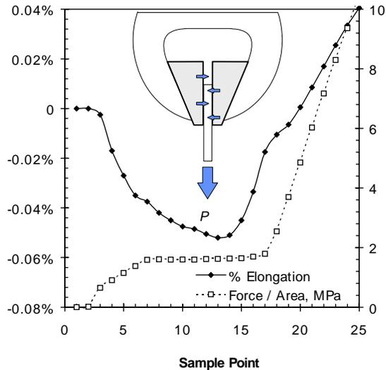
Figure 12: The Self-Tightening of the Wedge-Action Grips Was Considered to be Responsible for the Large Variability in Strain and Modulus Measurement (Figure 5)
