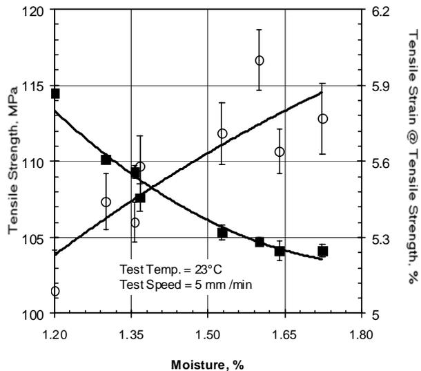
Figure 9: Change of tensile strength and tensile strain at tensile strength vs. moisture content for 33 wt% glass fiber reinforced polyamide 6
