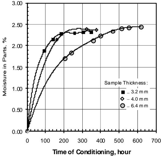
Figure 1: Moisture content vs. time of conditioning for 33 wt% glass fiber reinforced polyamide 6
