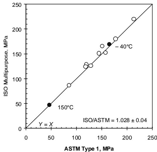
Figure 2: Tensile Strength of Materials,  $\sigma_M$ .  $T = 23^\circ\text{C}$  unless otherwise indicated
