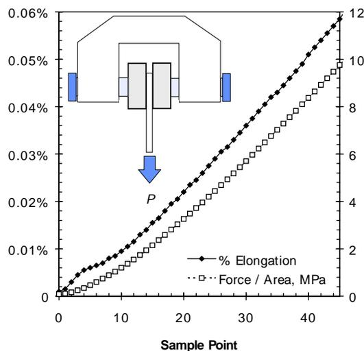
Figure 13: "Well-Behaved" Stress and Strain Curves with the Use of Side-Action Grips
