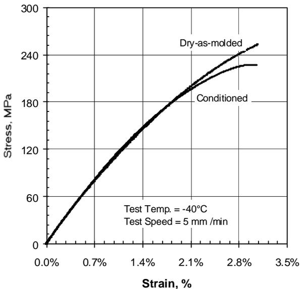
Figure 6: Tensile stress-strain curves at -40°C for 33 wt% glass fiber reinforced polyamide 6, dry-as-molded and
