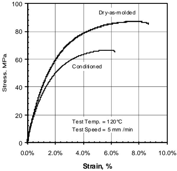
Figure 7: Tensile stress-strain curves at 120°C for 33 wt% glass fiber reinforced polyamide 6, dry-as-molded and conditioned
