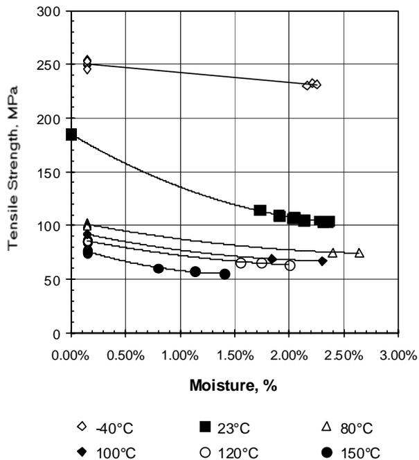
Figure 10: Tensile strength vs. moisture at different testing temperature for 33 wt% glass fiber reinforced polyamide 6
