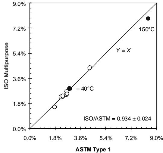
Figure 3: Tensile Strain at Tensile Strength,  $\epsilon_M$ . T = 23°C unless otherwise indicated
