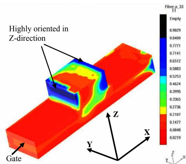
Figure 1. Predicted Z-direction fiber orientation: Flat Bump. Highest orientation seen at leading/trailing edges of center flat bump.
