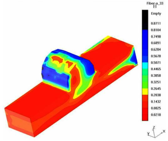
Figure 3. Predicted Z-direction fiber orientation: Round Bump.
