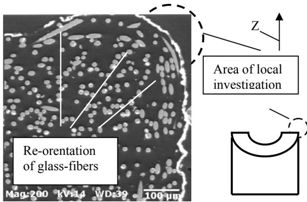
Figure 6. An example of localized and optimized glass-fiber orientation (for smooth groove, see Figure 4).
