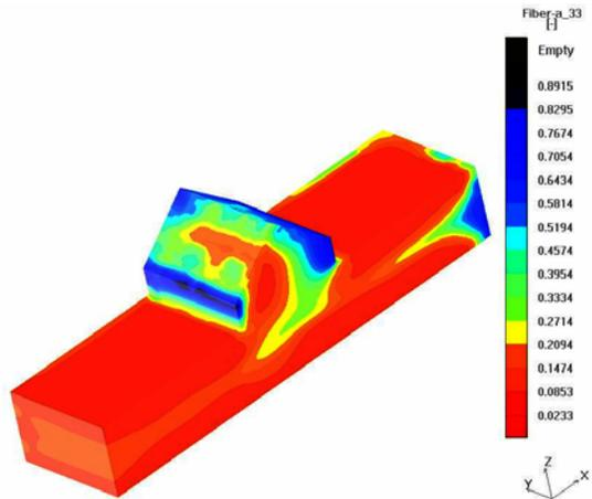
Figure 2. Predicted Z-direction fiber orientation: Tooth (similar to energy director). High orientation located at leading/trailing edges.
