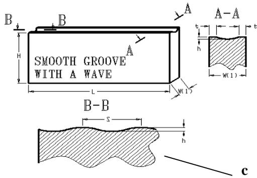
Figure 5. Principles of butt-joint geometry: a – flat configuration; b – an example of non-flat contact conditions (2-D presentation); c – waved geometry.
