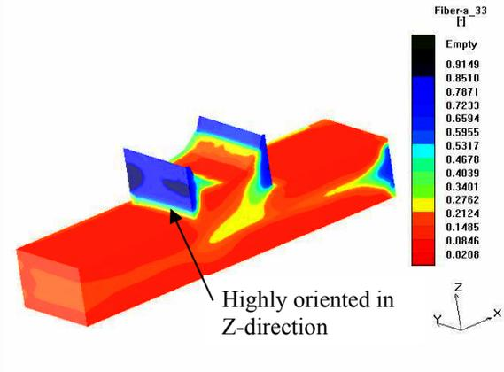
Figure 4. Predicted Z-direction fiber orientation: Smooth Groove
