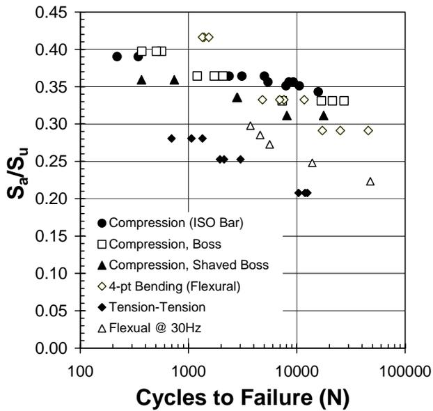
Figure 5. Master  $S_a/S_u - N_f$  Curve for All Fatigue Tests. Agenda: where  $S_a$  is stress amplitude;  $S_u$  is static strength of plastic/used specimen, and  $N_f$  is number of cycles to failure.
