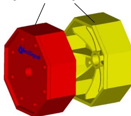
Figure 4. Multi-purpose universal welding & testing system. Consists from welded together two octagonal specimens (U.S. Patent # 6,193,133 [11]).
