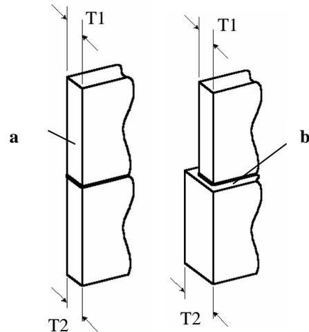
Figure 2. Principle of butt-joint geometry (a – similar, and b - dissimilar thickness welds)
