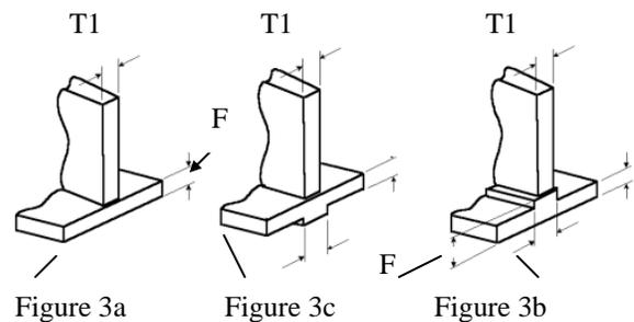
Figure 3 (a, b, c). Principles of T-type joint geometry (a – similar by thickness parts, b – with T-shape weld-bead, c – reverse position of Tr-shape weld-bead). **F** is the thickness of T-element at the future joint area.
