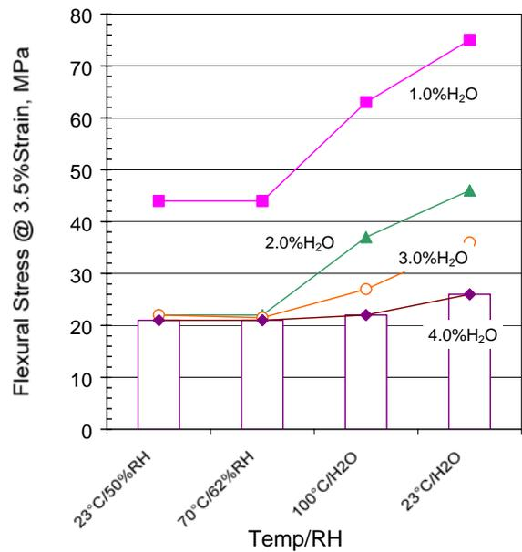
Figure 7. Effects of Conditioning Methods on Flexural Stress.
