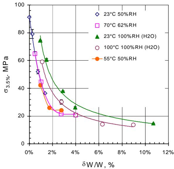
Figure 5. Flexural Stress @ 3.5% Flexural Strain vs. Moisture.
