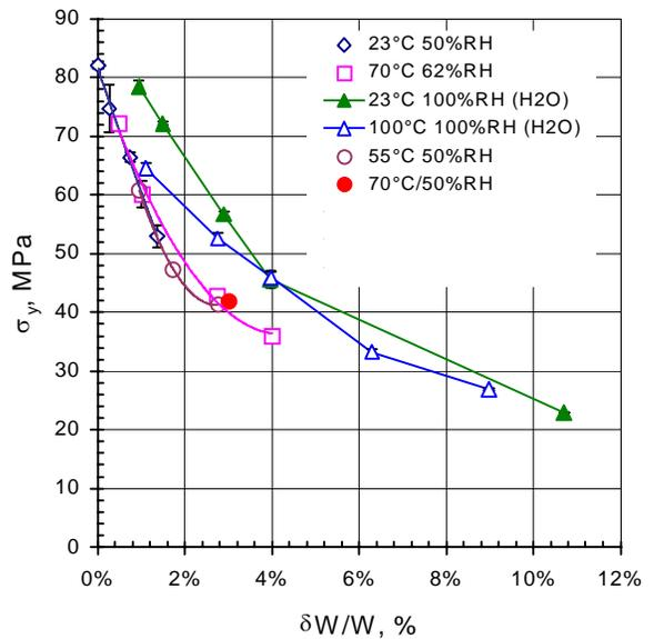
Figure 3. Tensile Stress at Yield vs. Moisture.
