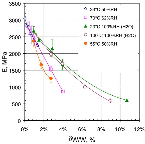
Figure 4. Tensile Modulus vs. Moisture.
