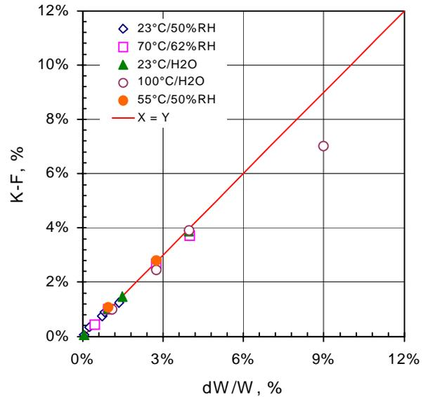
Figure 2. Efficiency of Moisture Measurement Methods: Weight change vs. Karl-Fischer
