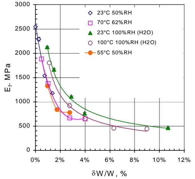
Figure 6. Flexural Modulus vs. Moisture.
