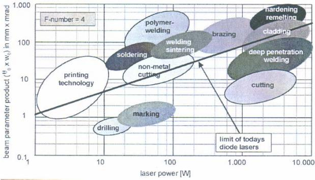
Figure 6 Relations between laser beam quality and power.
