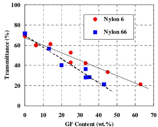
Figure 4. Transmittance of nylon 6 vs. nylon 66 based plastics (natural state) with the influence of fiberglass reinforcement at 830 nm. Specimen Thickness is 3.2mm.
