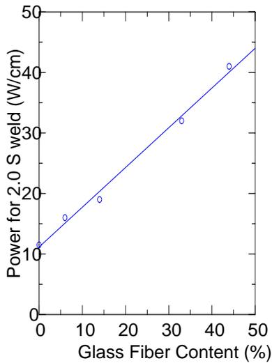
Figure 7. Influence of glass-fiber reinforcements (in %, for nylon 6, part thickness = 3.2 mm) on power requirement to make a weld in 2.0 S. Legend: short fiber-glass reinforcement from 6 wt. % to 45 wt. %.
