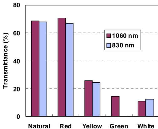
Figure 2. Influence of wavelength (at 830 and 1060 nm) on transmittance ( $T$ ) properties for the following versions of colored nylon: red, yellow, green, white and natural. The thickness of the specimens is 3.2 mm.
