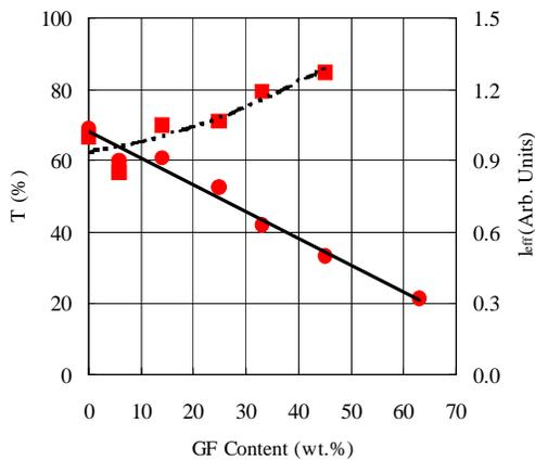
Figure 1. Transmittance ( $T$ ) and effective pathlength ( $l_{\text{eff}}$ ) at wavelength  $1.06 \mu\text{m}$  of nylon 6 with the influence of fiber-glass (GF) content (wt. %). Effective pathlength is normalized to 1.0 at 0 wt. % GF content). Thickness of the specimens is 3.2 mm.
