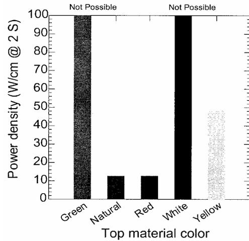
Figure 9. Power density needed to weld different colored un-filled nylon 6 specimens (thickness = 3.2 mm).
