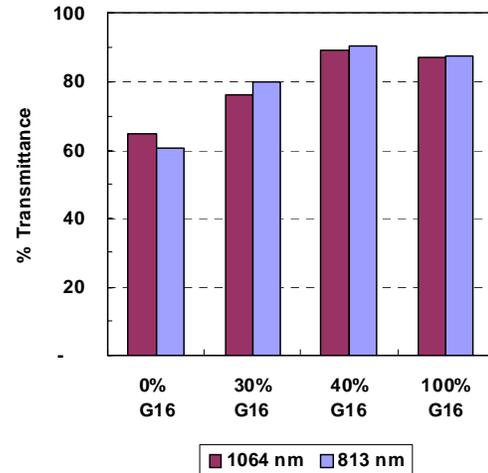
Figure 3. Influence of wavelength (at 1064 and 813 nm) on transmittance ( $T$ ) properties for the blends of nylon 6 (Capron® un-filled grade) with amorphous nylon (Grivory®<sup>7</sup> grade). Thickness of the specimens is 3.2mm. Color version: natural state.
