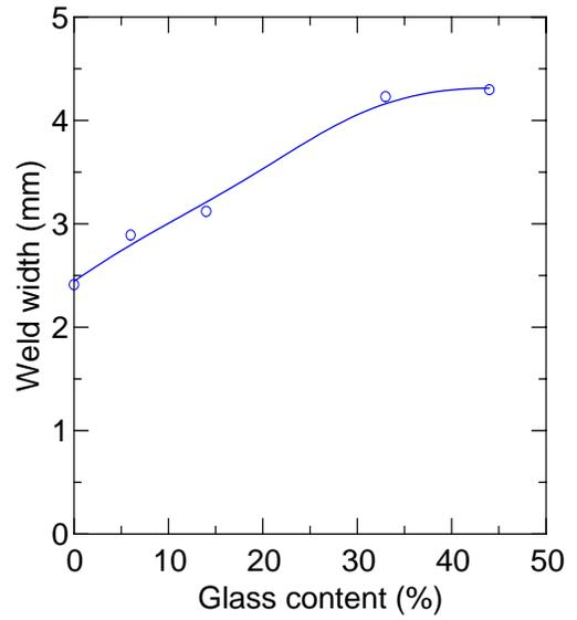
Figure 8. Effects of fiber-glass content (in %) on weld width (in mm for nylon 6, part thickness = 3.2 mm). Legend: short fiber-glass reinforcement from 6 wt. % to 45 wt. %.
