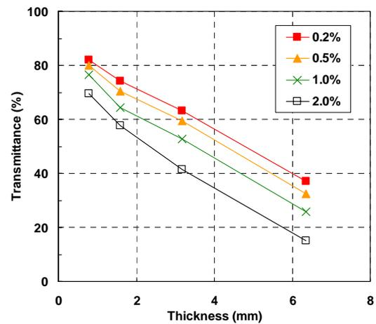
Figure 3: Influence of thickness on transmission (1064 nm) of unfilled, black colored (0.25 to 2 wt %) PA 6.
