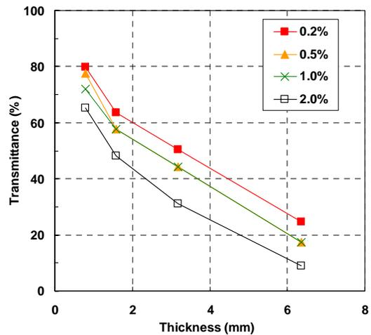
Figure 4: Influence of thickness on transmission (830 nm) of unfilled, black colored (0.25 to 2 wt %) PA 6.
