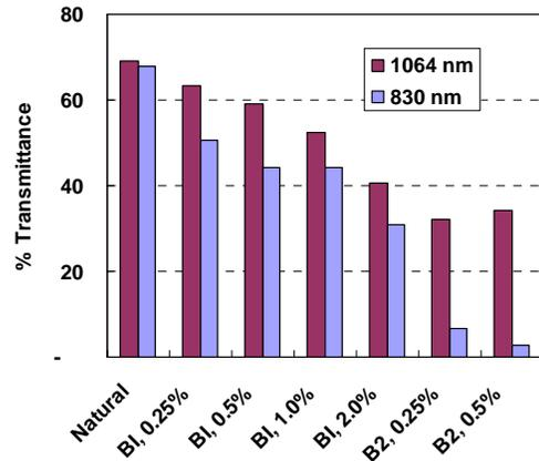
Figure 2. Influence of wavelength (830 and 1,064 nm), type of colorant and colorant concentration on the transmittance of unfilled PA 6. Specimen thickness is 3.2mm. Color version: non-carbon black.
