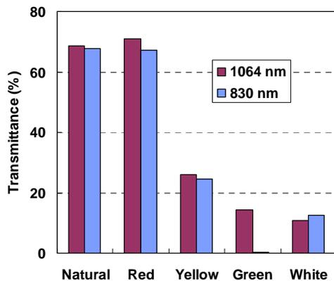
Figure 1. Influence of wavelength (at 830 and 1,064 nm) on transmittance for colored (red, yellow, green, white, natural) PA 6 plastics. Specimen thickness is 3.2 mm.
