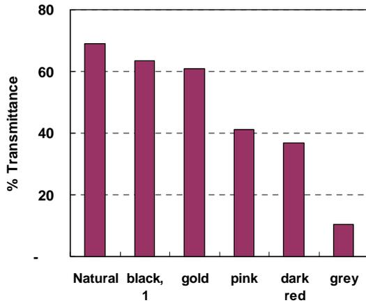
Figure 5. Efficiency of “*J – Technology*” on the transmittance of the various colored PA 6 plastics (at the wavelength 1.06 μm). Sample thickness is 3.2 mm. Color versions: natural state, gold, pink, dark red and gray.
