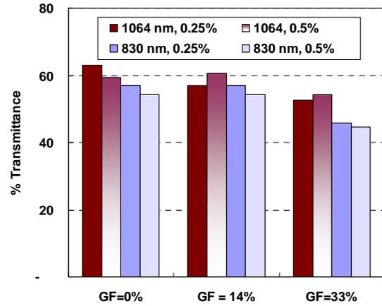
Fig. 6: Influence of wavelength (830 and 1,064 nm) and fiber-glass (GF) reinforcement (14 and 33 wt.%) on laser transmission of black PA 6 plastics. Thickness of the specimens is 3.2mm. Color version: black type B (non-carbon black). Legend gives colorant concentration.
