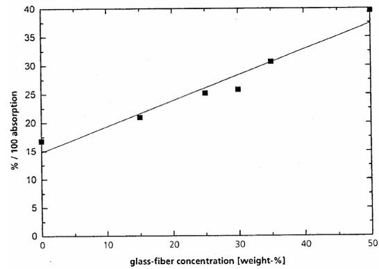
Figure 4. Absorption properties ( $A$ ) of PA with the influence of fiberglass reinforcement (0-50 wt.% GF).
