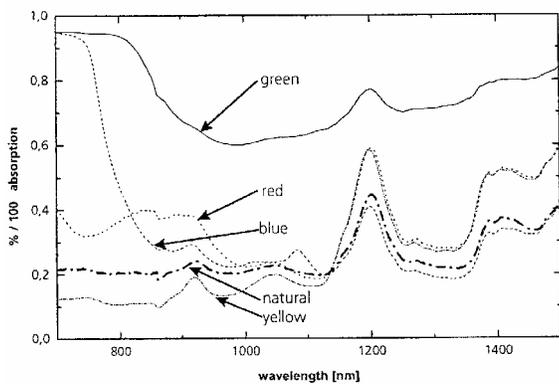
Figure 2. Influence of wavelength on absorption ( $A$ ) properties for the following versions of colored PA: green, red, blue, natural and yellow.
