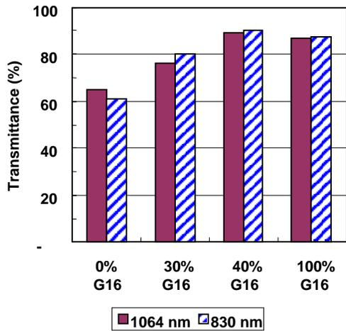
Figure 6. Influence of wavelength (at 1,064 and 830 nm) on transmittance ( $T$ ) properties for the blends of PA 6 with amorphous PA (G 16).
