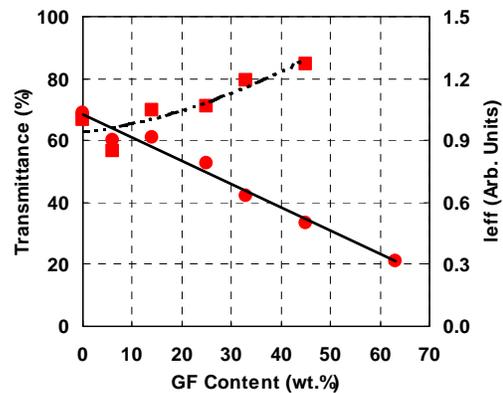
Figure 5. Transmittance ( $T$ ) at 1,064 nm and effective pathlength ( $l_{eff}$ ) of PA 6 plastics with the influence of fiberglass (GF) content (wt. %). Effective pathlength ( $l_{eff}$ , normalized to 1.0 at 0% GF content).
