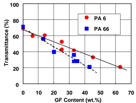
Figure 9. Transmittance of PA 6 vs. PA 66 based plastics with the influence of fiber-glass reinforcement (at wavelength 830 nm). Thickness of the specimens is 3.2mm. Color version: natural state
