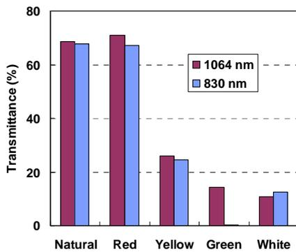
Figure 7. Influence of wavelength (at 830 and 1,064 nm) on transmittance ( $T$ ) properties for the following versions of colored PA: red, yellow, green, white and natural. Thickness of the specimens is 3.2 mm.
