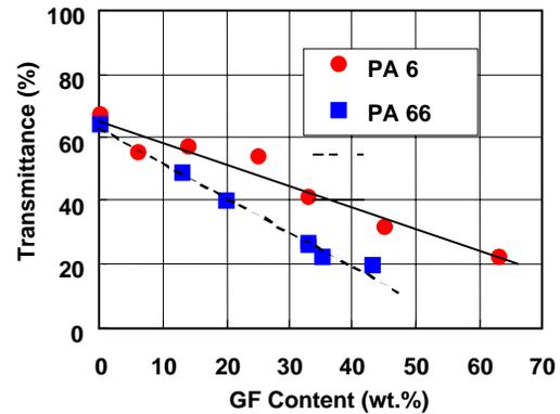
Figure 8. Transmittance of PA 6 vs. 66 based plastics with the influence of fiberglass reinforcement (at wavelength 1,064 nm). Thickness of the specimens is 3.2mm. Color version: natural state.
