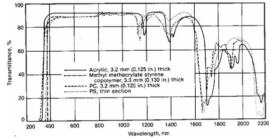
Figure 3. Influence of wavelength on transmittance ( $T$ ) for four optical plastics.
