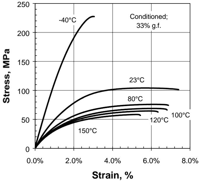
Figure 5b. Effect of temperature on tensile behavior of conditioned nylon 6 (33% glass fiber).
