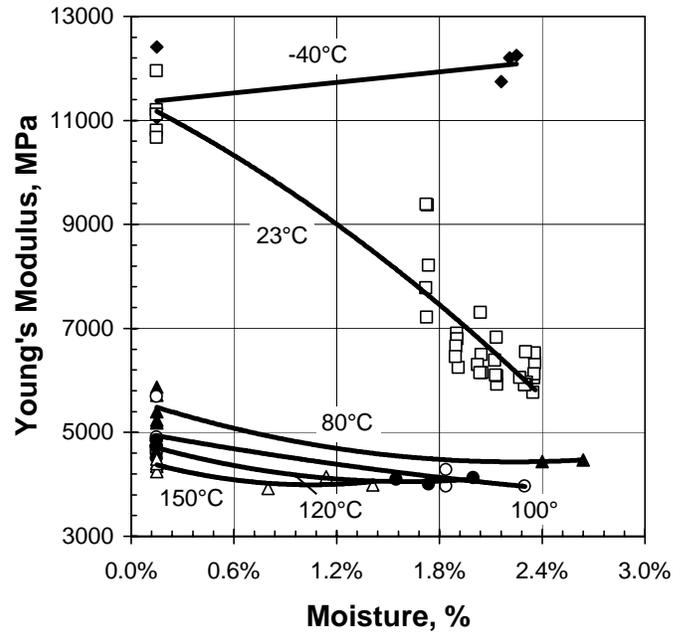
Figure 9. Impact of temperature and moisture on Young's modulus of reinforced nylon 6 (33% glass fiber).
