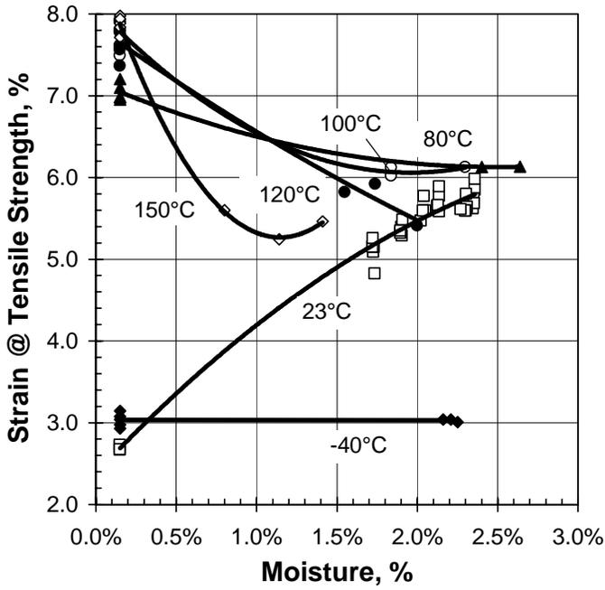
Figure 8. Impact of temperature and moisture on tensile strain @ tensile strength of reinforced nylon 6 (33% glass fiber).
