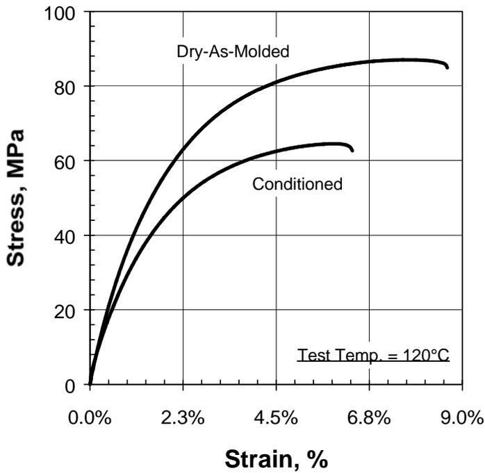
Figure 2c. Effect of moisture on tensile behavior of reinforced nylon 6 (33% glass fiber) at elevated temperature.
