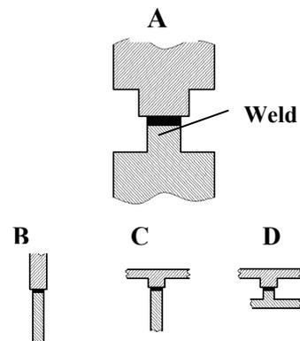
Figure 2: Welded joint design principles (types and configuration). Legend: A – joint design; B – butt joint (straight); C – butt joint (T – shape); D – shear / lap joint
