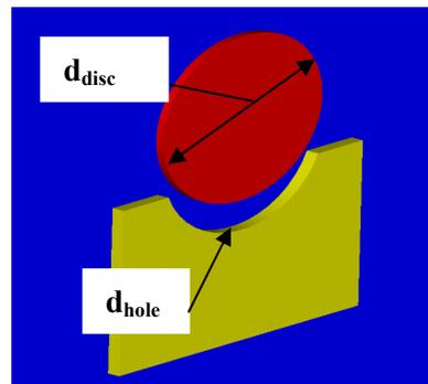
Figure 8: Curvilinear model of the welded joint (injection molded disc and plaque will be joined together by linear vibration welding)
