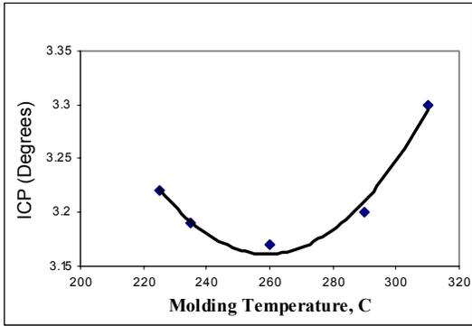
Figure 12: Influence of molding / melt temperatures on ICP
