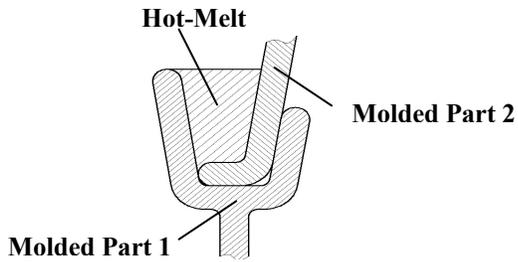
Figure 13: Principles of Hot-Melt joining (over-molding)
