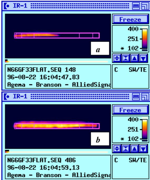
Figure 9: Temperature distribution in weld inter-phase (butt joint, nylon 66). *a* - heating initiation phase; *b* - at final phase of heating
