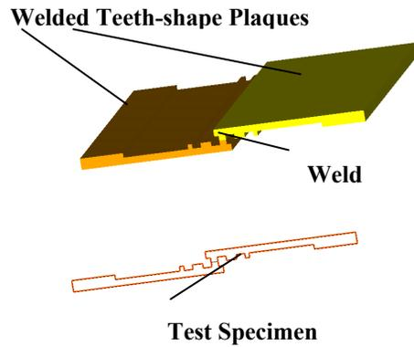
Figure 7: Model of welded shear / lap joint (consists from two teeth-shape injection molded plaques welded together. For teeth-element thickness of the weld beads are: 6; 4 and 2,5 mm)
