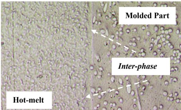
Figure 14: Joint Structure at Optimized Over-Molding Conditions
