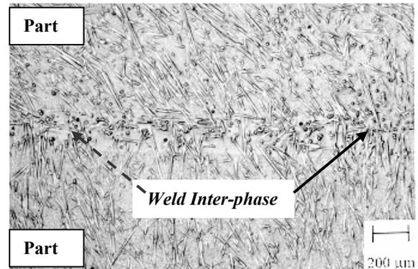
Figure 1: Local reinforcement effects at the weld inter-phase (a part of fibers are crossing the weld inter-phase)
