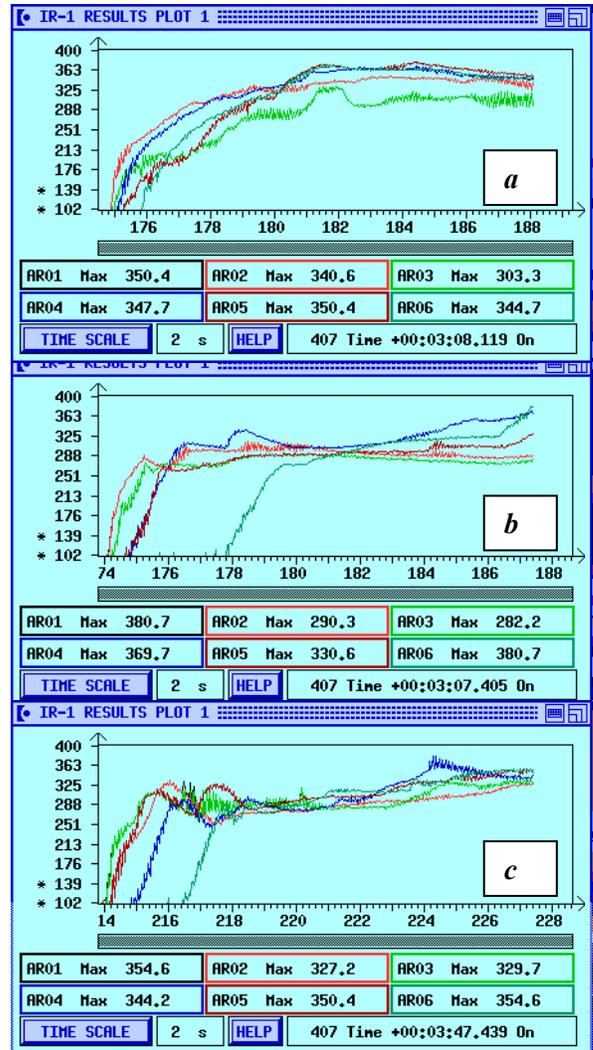
Figure 10: Time-temperature profiles (optimized LVW conditions, butt joint, and nylon 66). Type of plastics: *a* - non-reinforced / non-filled; *b* - 33 wt.% fiberglass reinforced; *c* - fiberglass reinforced and mineral filled.
