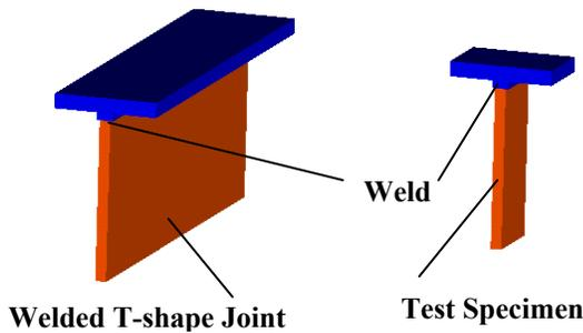
Figure 5: Model of welded T-shape butt joint (consists from welded together T-element and molded plaques. For T-element thickness of the weld bead is 6 mm. Thickness
