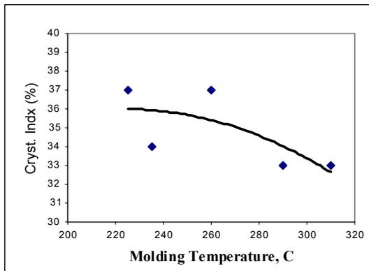
Figure 11: Influence of molding / melt temperatures on CI (crystallinity index)
