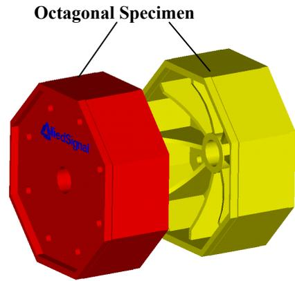
Figure 6: Multi-purpose universal welding & testing system (consists from welded together two octagonal specimens. Thickness of weld beads is: 6; 5; 4 and 2,5 mm)
