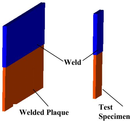
Figure 4: Model of welded straight butt joint (consists from two molded plaques welded together. Thickness of plaques is 6 mm and 4 mm) and machined / cut test specimen (width = 10 mm)
