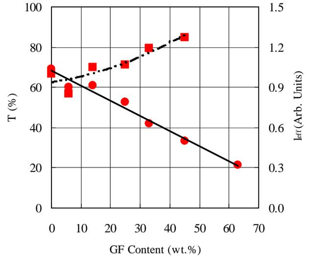
Figure 5: Effect of fiber-glass (GF) content (wt. %) on laser transmission (T) at 1.06  $\mu\text{m}$  compared to effective pathlength ( $l_{\text{eff}}$ , normalized to 1.0 at 0% GF content). Sample thickness is 3.2 mm.
