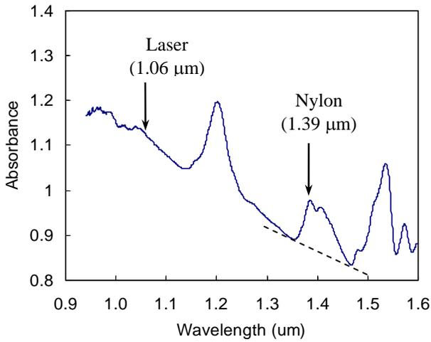
Figure 4: Representative NIR spectrum of a natural nylon 6 plaque (sample thickness = 3.2  $\mu\text{m}$ ). The nylon peak absorbance at 1.39  $\mu\text{m}$  is measured from the baseline (----) drawn from 1.33 to 1.47  $\mu\text{m}$
