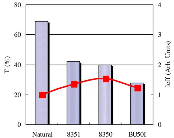
Fig. 10: Effect of impact modifier type (see Table 5) on laser transmission (T) at 1.06  $\mu\text{m}$  compared to effective pathlength ( $l_{eff}$ , normalized to 1.0 for Natural sample). Sample thickness is 3.2 mm.
