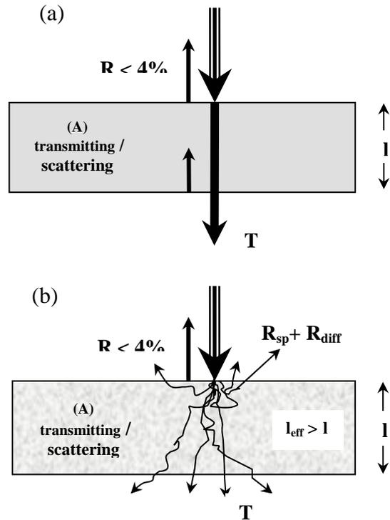
Figure 2: Transmission through plastic samples: (a) homogeneous, glass-like plastics; (b) inhomogeneous, semi-crystalline plastics.
