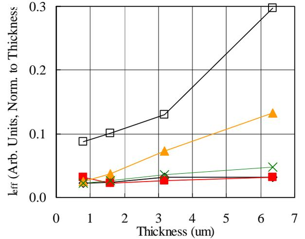
Fig. 9: Effect of plaque thickness and color version on the effective pathlength ( $l_{eff}$ , normalized to the thickness) for (natural) nylon 6 materials. Legend: natural ( $\diamond$ ); red ( $\blacksquare$ ); yellow ( $\square$ ); green (x); white ( $\square$ )
