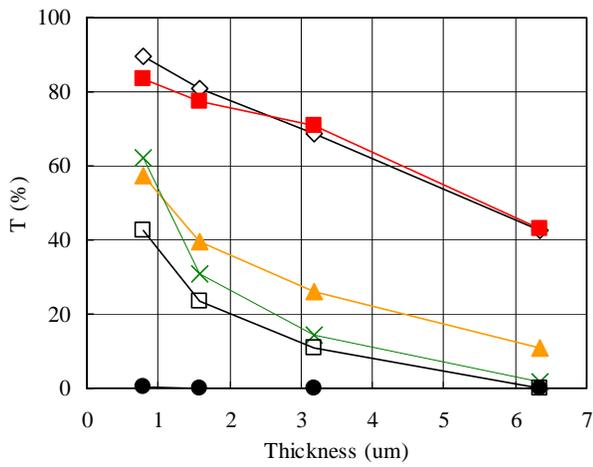
Figure 8: Effect of plaque thickness and color version on laser transmission (T) at 1.06  $\mu\text{m}$ . Legend: natural ( $\diamond$ ); red ( $\blacksquare$ ); yellow ( $\square$ ); green (x); white ( $\square$ ); black ( $\bullet$ )
