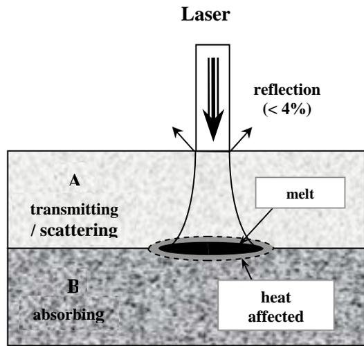
Figure 1: Principle of the laser transmission welding. Part A is a thermoplastic having variable transmission/ scattering. The thermoplastic in part B absorbs the transmitted light at the interfacial region
