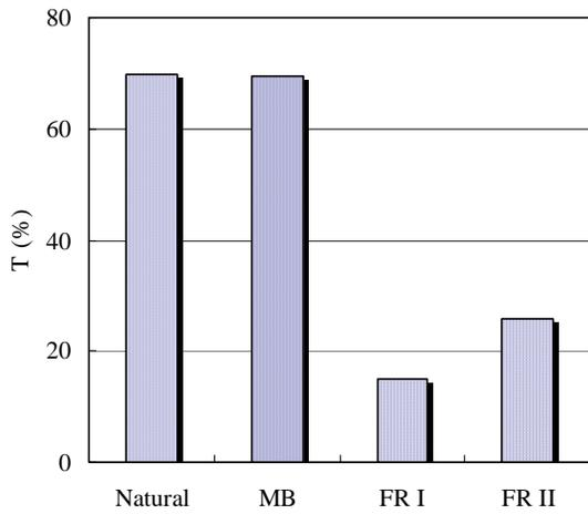
Fig. 12: Effect of maserbatch and flame retardant additives on laser transmission (T) at  $1.06 \mu\text{m}$ . Sample thickness is 3.2 mm, except for FR I and II (1.6 mm).
