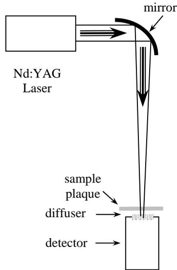
Figure 3: Apparatus for measuring laser transmission at 1.06  $\mu\text{m}$
