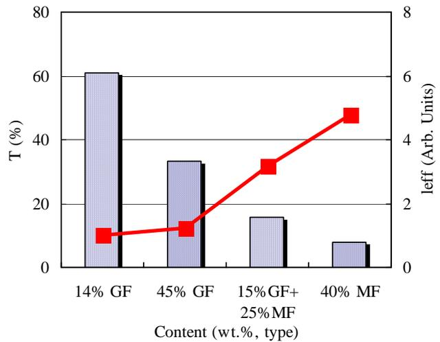
Figure 6: Effect of fiber-glass (GF), mineral filler (MF) and content (wt. %) on laser transmission (T) at 1.06  $\mu\text{m}$  compared to effective pathlength ( $l_{\text{eff}}$ , normalized to 1.0 at 14% GF content). Sample thickness is 3.2 mm.
