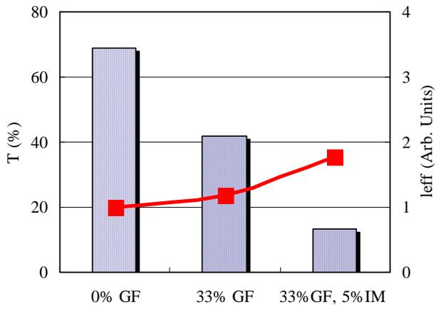
Fig. 11: Combined effect of impact modifier and fiber-glass reinforcement (Table 4) on laser transmission (T) at  $1.06 \mu\text{m}$  compared to effective pathlength ( $l_{eff}$ , normalized to 1.0 for Natural sample). Sample thickness is 3.2 mm.
