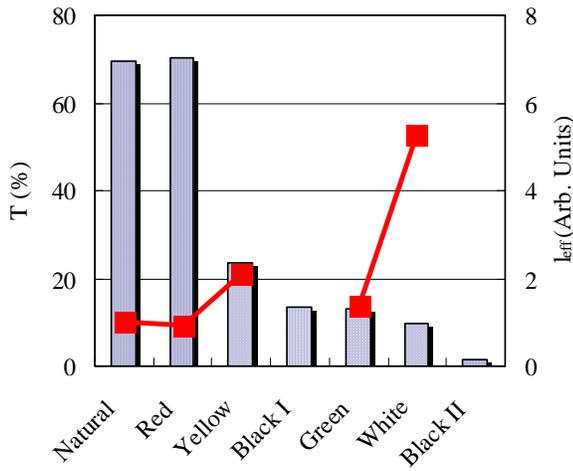
Figure 7: Effect of color version on laser transmission (T) at 1.06  $\mu\text{m}$  compared to effective pathlength ( $l_{eff}$ , normalized to 1.0 for Natural sample). Sample thickness is 3.2 mm.
