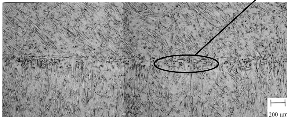
Fig. 7: Fiber-Glass Orientation at Optimized LVW Conditions (Local Reinforcement Effects in Weld Inter-phase)
