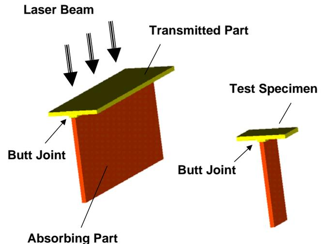
Figure 15: T-type joint for the laser transmission welding (LTW)
