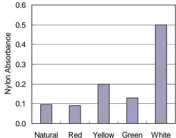
Figure 9: Influence of color version on nylon absorbance at 1.39  $\mu\text{m}$  (sample thickness = 3.2 mm)
