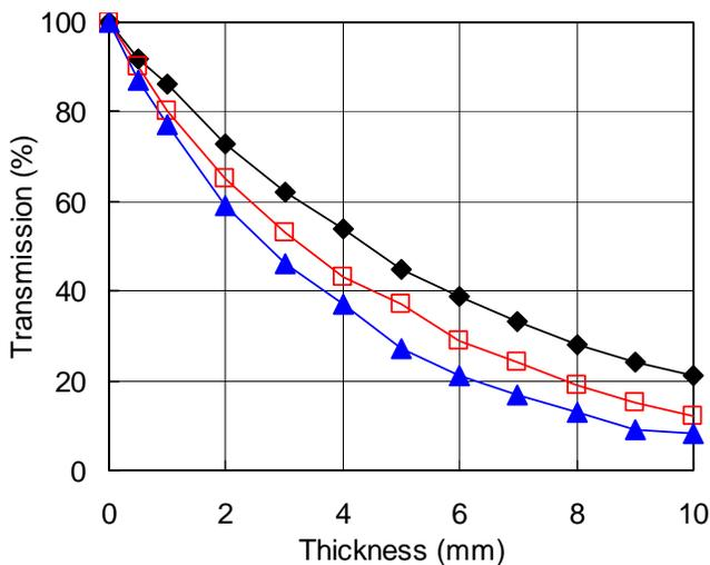
Figure 10: Influence of thickness on laser transmission of semi-crystalline non-colored (natural) plastics at 1.06  $\mu\text{m}$ . Legend: PA ( $\blacklozenge$ ); HDPE ( $\square$ ); PP ( $\blacktriangle$ ) [33]
