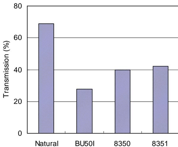
Fig. 13: Influence of impact modifier type (see Table 2) on laser transmission at 1.06 μm for natural nylon 6 (sample thickness = 3.2 mm)
