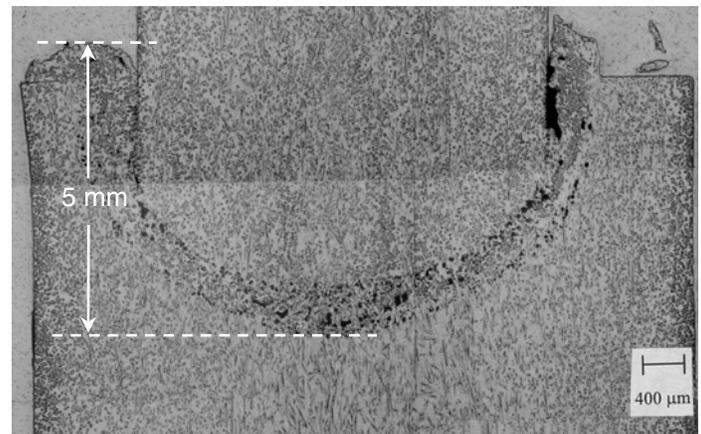
Figure 16: Wide gap adjustment for linear vibration welding (LVW): nylon 6, 33GF wt.% (longitudinal oscillations, melt-down = 5 mm)
