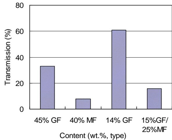
Figure 6: Influence of fiber-glass (GF), mineral filler (MF) and content (wt.%) on laser transmission at 1.06  $\mu\text{m}$  (sample thickness = 3.2 mm)
