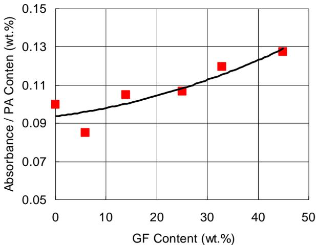
Figure 5: Influence of fiber-glass content (wt.%) on nylon absorbance at 1.39  $\mu\text{m}$  (normalized to nylon 6 content), (sample thickness = 3.2 mm)
