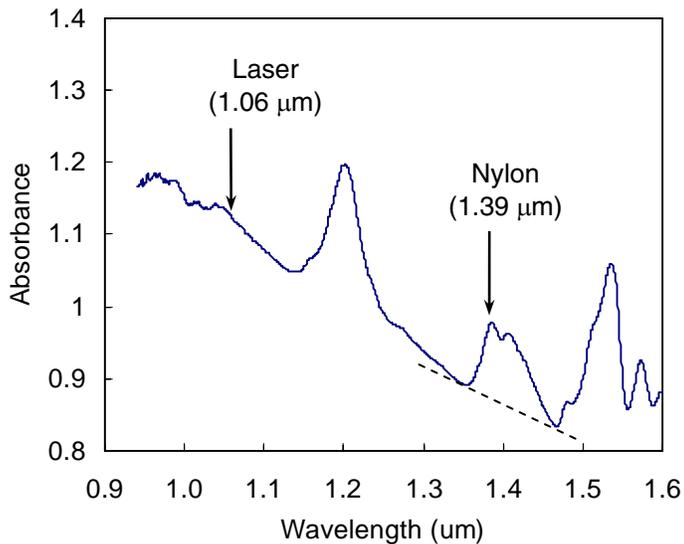
Figure 3: Representative NIR spectrum of a natural nylon 6 plaque (sample thickness = 3.2 µm). The nylon peak absorbance at 1.39 µm is measured from the baseline (-----) drawn from 1.33 to 1.47 µm
