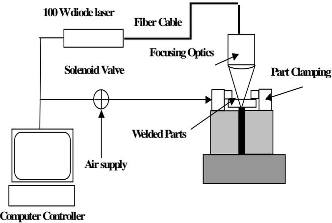
Figure 20: Set-up for laser transmission welding machine
