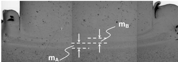
Figure 18: Butt joint structure for laser transmission welding of nylon 6 based plastics. Legend:  $m_A$  – melt layer thickness of the weld related to laser transmitting plastic;  $m_B$  – melt layer thickness of the weld related to absorbing plastic
