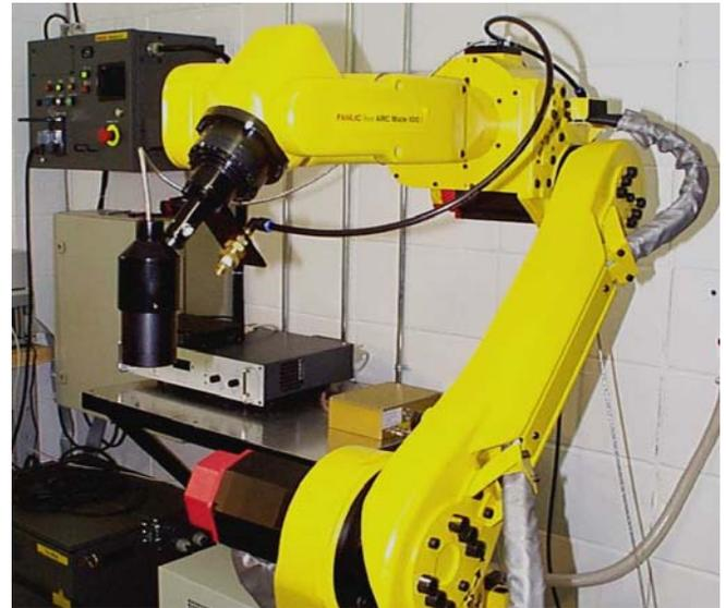
Figure 21: Laser transmission welding (LTW) machine with complete robotic system
