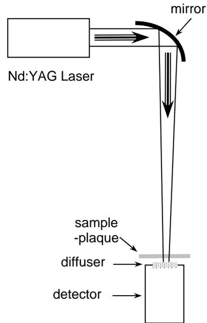
Figure 2: Apparatus for measuring laser transmission at 1.06  $\mu\text{m}$
