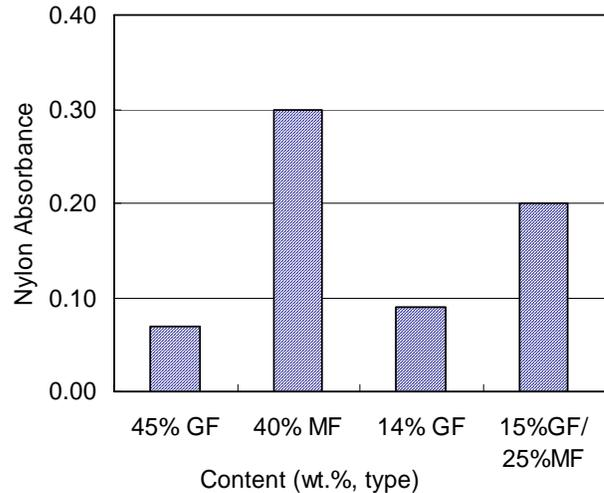
Figure 7: Influence of fiber-glass (GF), mineral filler (MF) and content (wt.%) on nylon absorbance at 1.39  $\mu\text{m}$  (sample thickness = 3.2 mm). The absorbance for natural nylon 6 is 0.10
