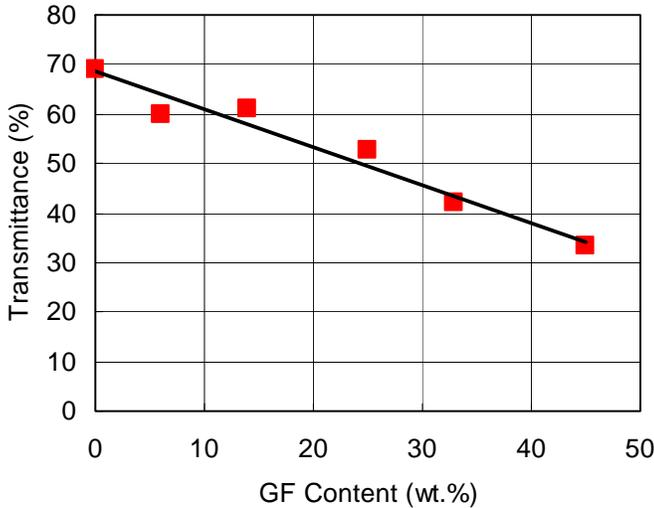
Figure 4: Influence of fiber-glass content (wt.%) on laser transmission at 1.06  $\mu\text{m}$  (sample thickness = 3.2  $\mu\text{m}$ )
