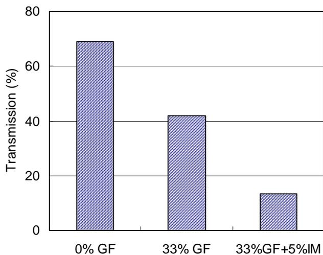
Fig. 14: Combined influence of impact modifier and fiber-glass reinforcement (see Table 2) on laser transmission at 1.06 μm for nylon 6 (sample thickness = 3.2 mm)
