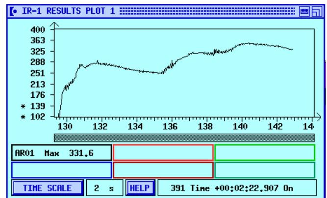
Figure 23: Time-temperature profile for welding of 33wt.% fiber-glass reinforced nylon 6 plastic
