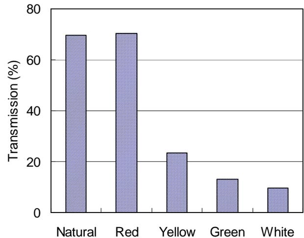
Figure 8: Influence of color version on laser transmission at 1.06  $\mu\text{m}$  (sample thickness = 3.2 mm)
