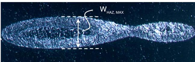
Figure 22: Weld and melt-pool profile for a lap / shear joint (See Table 4)
