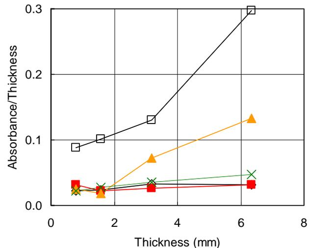
Fig. 12: Influence of thickness on the effective pathlength for (natural) nylon 6 measured by the nylon absorbance (normalized to thickness) at 1.39  $\mu\text{m}$ . Legend: natural ( $\diamond$ ); red ( $\blacksquare$ ); yellow ( $\square$ ); green ( $\times$ ); white ( $\square$ )
