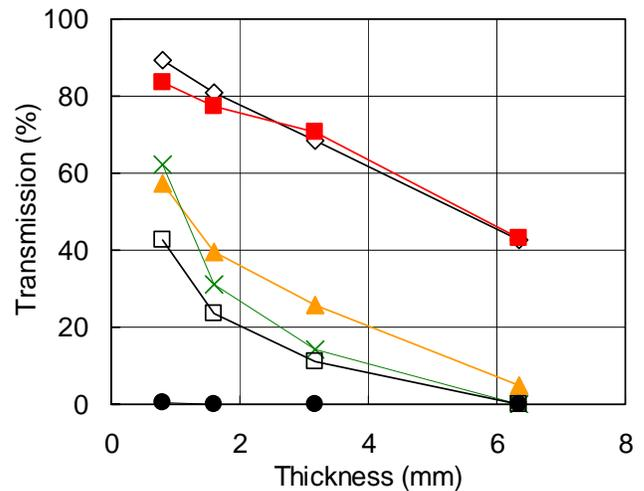
Figure 11: Influence of plaque thickness and color version on laser transmission at 1.06  $\mu\text{m}$ . Legend: natural ( $\diamond$ ); red ( $\blacksquare$ ); yellow ( $\square$ ); green ( $\times$ ); white ( $\bullet$ )
