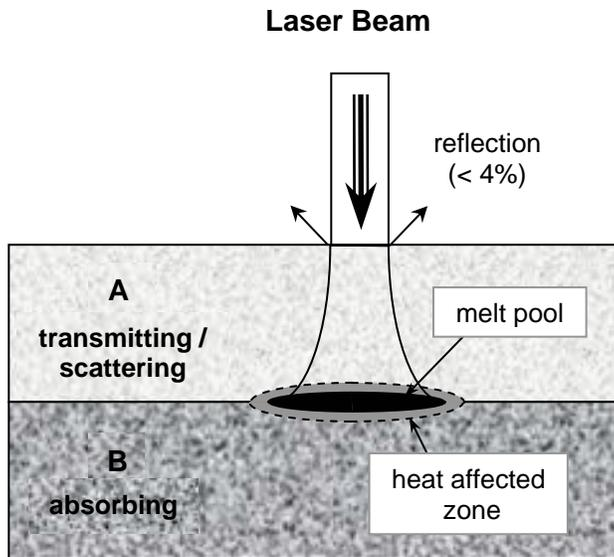
Figure 1: Principle of the laser transmission welding. Part A is a thermoplastic having variable transmission/scattering. The thermoplastic in part B absorbs the transmitted light at the interfacial region
