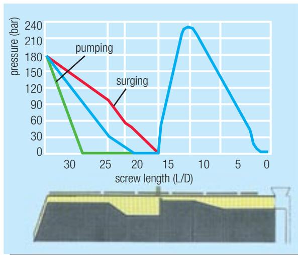
**Fig. 12:** Pressure variation in a degassing screw.
