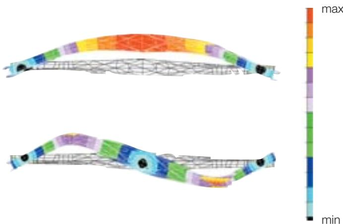
**Fig. 5:** Stabilizer link made of Ultramid®; deformation beyond buckling load; top: 1. eigenmode, bottom: 3. eigenmode.
