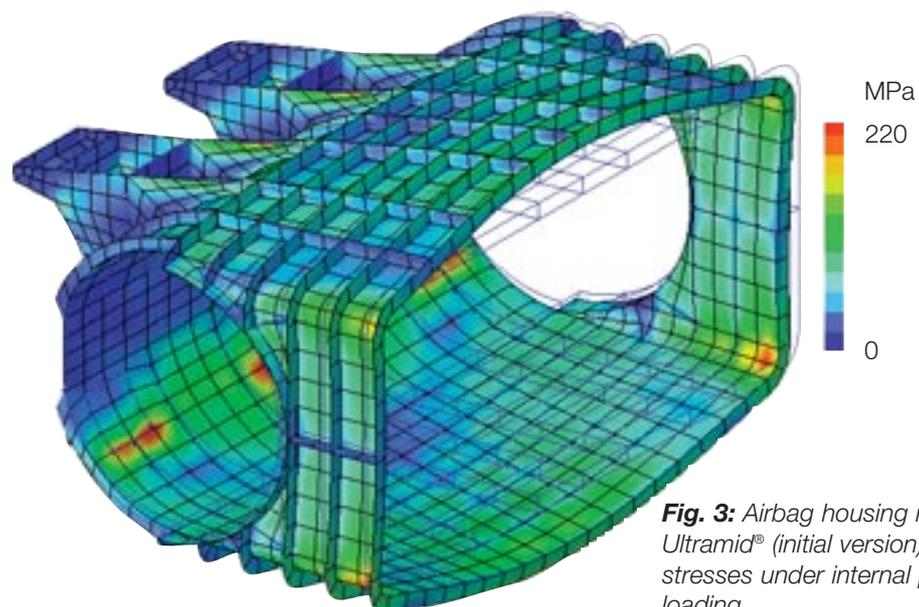
**Fig. 3:** Airbag housing made of Ultramid® (initial version); effective stresses under internal pressure loading.
