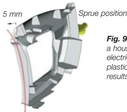
**Fig. 9a:** Warpage of a housing of an electrical tool; left: plastic part; right: results of simulation.
