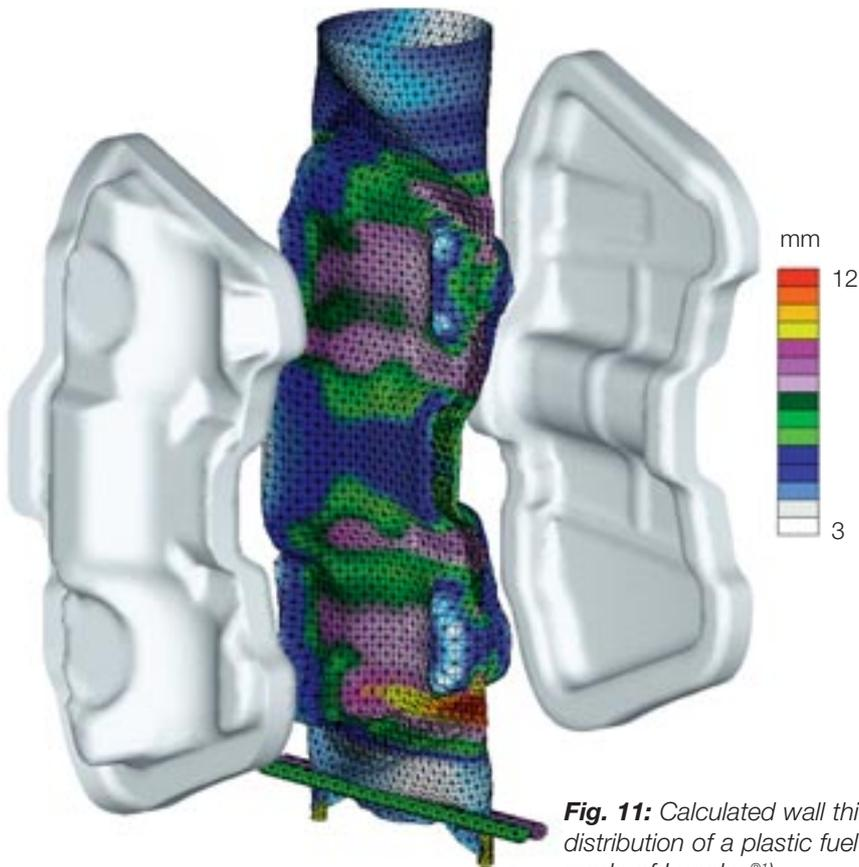
**Fig. 11:** Calculated wall thickness distribution of a plastic fuel tank made of Lupolen<sup>®1</sup>.
