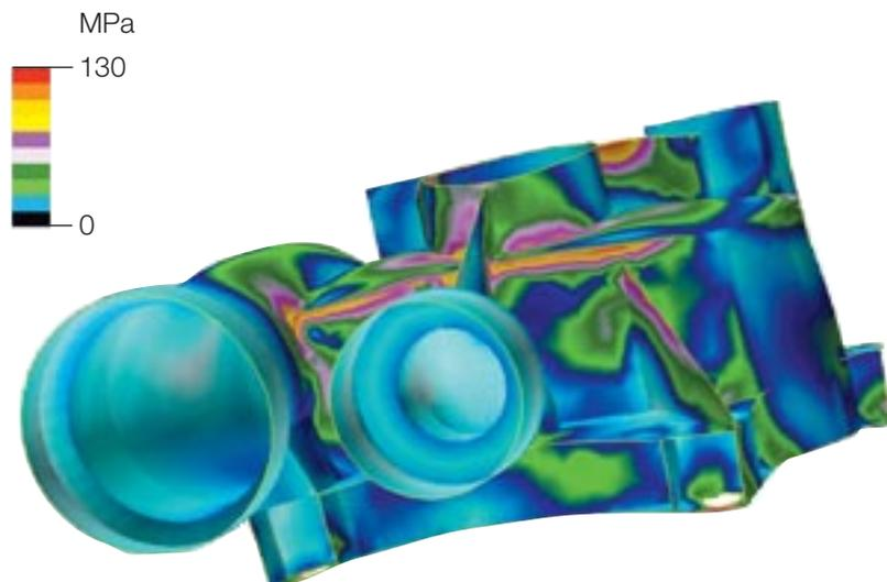
**Fig. 2:** Deformation of an Ultramid® housing (automotive gear shift) under excessive load.
