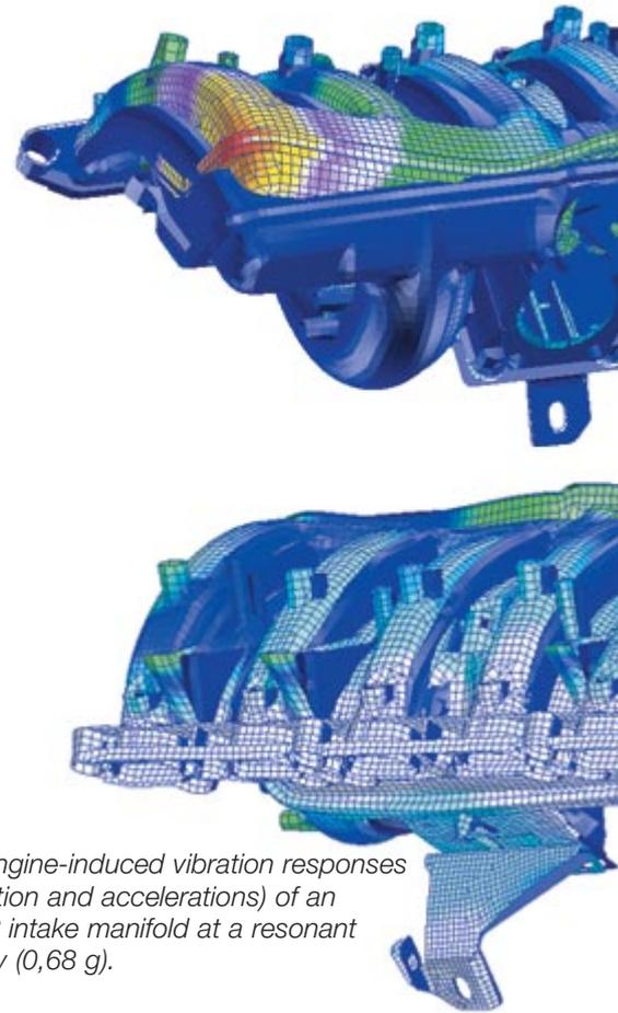
**Fig. 6:** Engine-induced vibration responses (deformation and accelerations) of an Ultramid® intake manifold at a resonant frequency (0,68 g).
