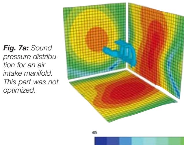
**Fig. 7a:** Sound pressure distribution for an air intake manifold. This part was not optimized.
