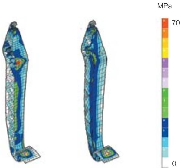
**Fig. 4:** Ultramid® clutch pedal. Left: initial version; right: version optimized for rigidity and strength; effective stresses under test load.
