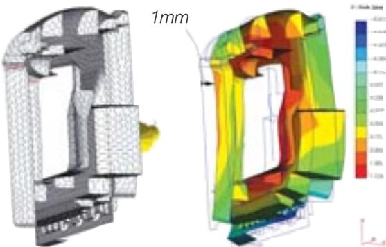
**Fig. 9b:** Fibre orientation and warpage analysis for the part shown in fig. 9a with changed sprue position.
