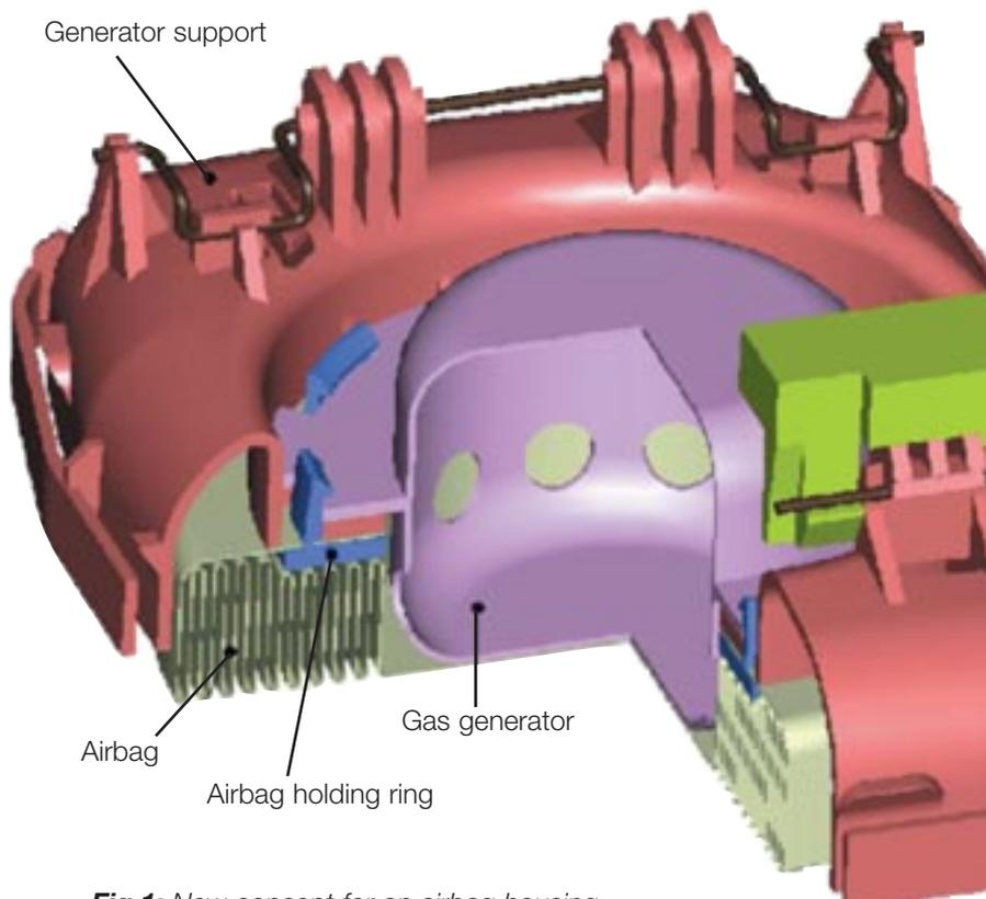
**Fig.1:** New concept for an airbag housing, integrated into the steering-wheel.
