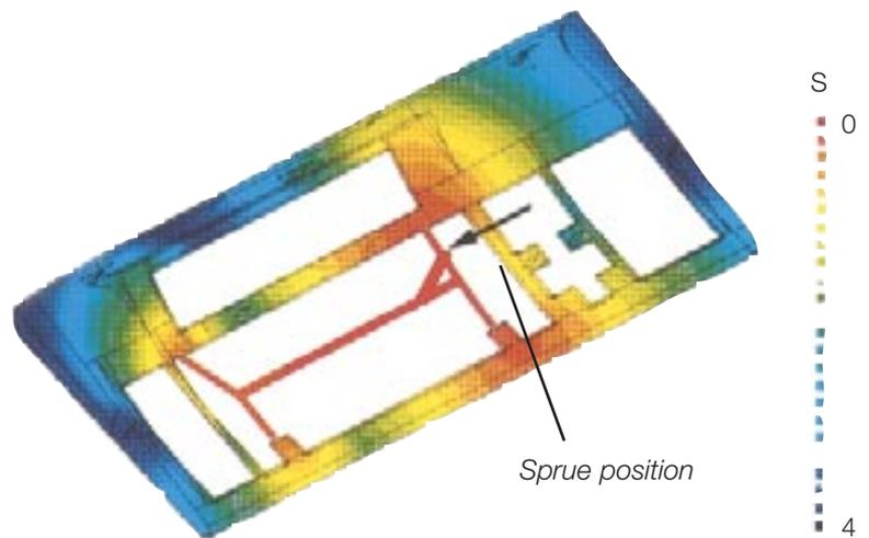
**Fig. 8:** Melt flow pattern of the upper part of a keyboard.
